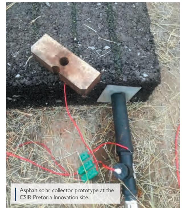
Asphalt solar collector prototype at the CSIR Pretoria Innovation site.
