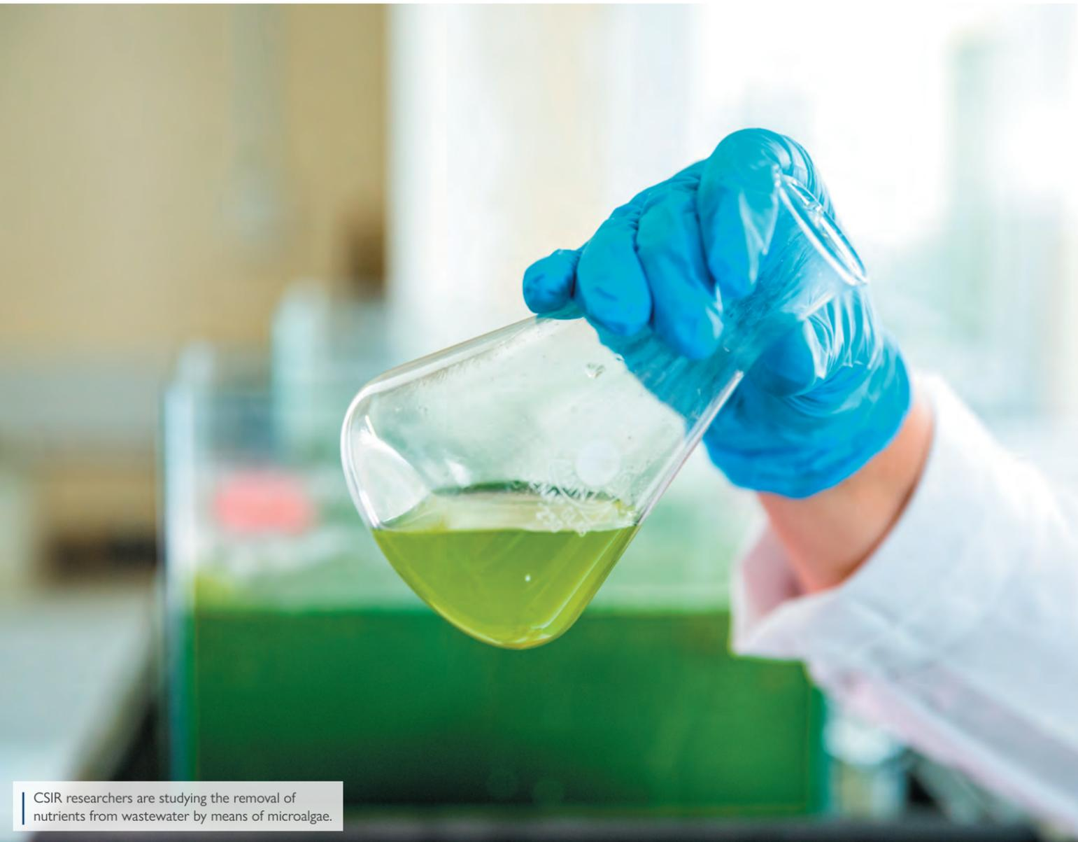
CSIR researchers are studying the removal of nutrients from wastewater by means of microalgae.
