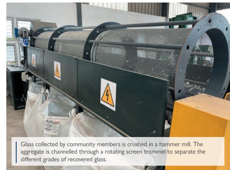
Glass collected by community members is crushed in a hammer mill. The aggregate is channelled through a rotating screen trommel to separate the different grades of recovered glass.
