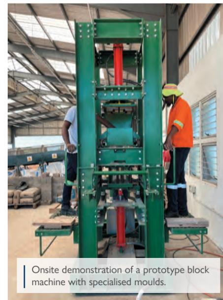
Onsite demonstration of a prototype block machine with specialised moulds.
