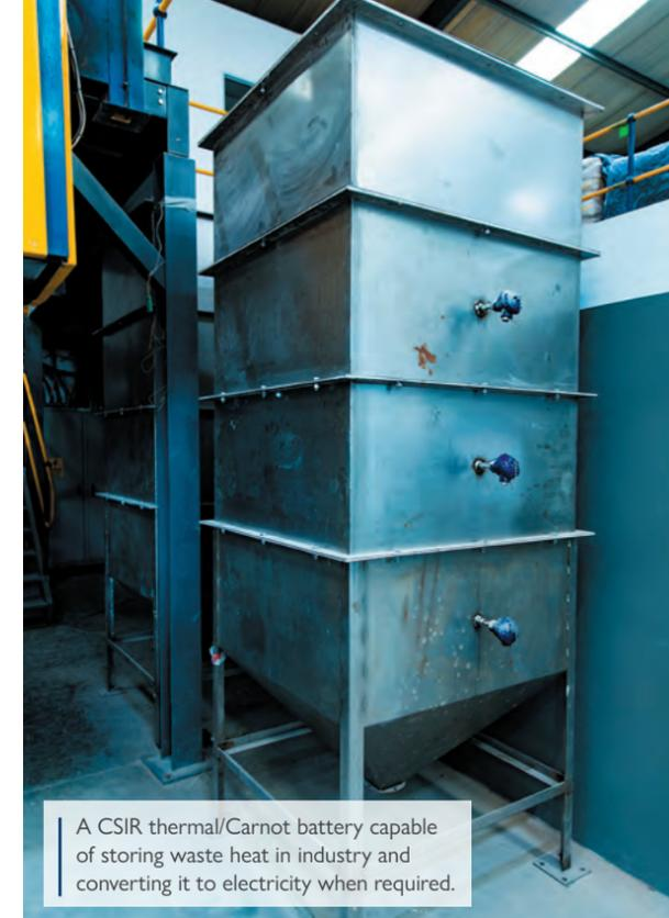
A CSIR thermal/Carnot battery capable of storing waste heat in industry and converting it to electricity when required.
