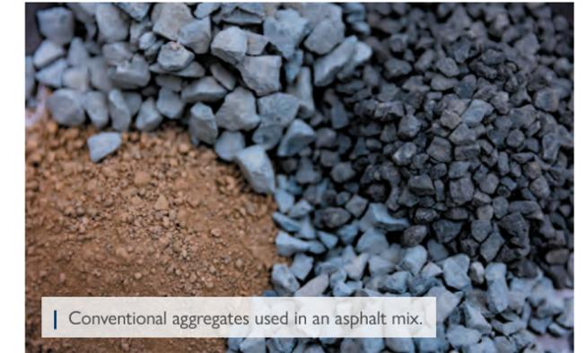
Conventional aggregates used in an asphalt mix.
