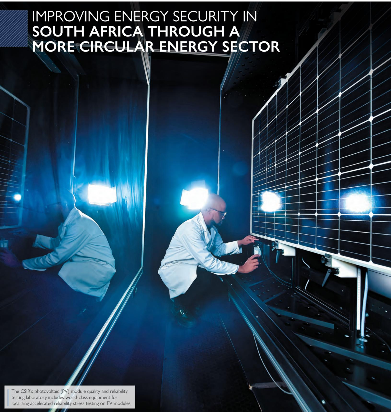
The CSIR's photovoltaic (PV) module quality and reliability testing laboratory includes world-class equipment for localising accelerated reliability stress testing on PV modules.
