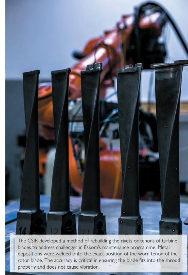
The CSIR developed a method of rebuilding the rivets or tenons of turbine blades to address challenges in Eskom's maintenance programme. Metal depositions were welded onto the exact position of the worn tenon of the rotor blade. The accuracy is critical in ensuring the blade fits into the shroud properly and does not cause vibration.
