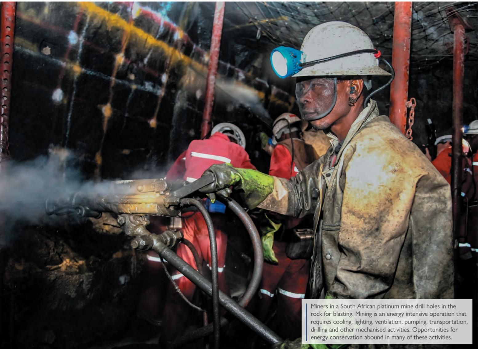
Miners in a South African platinum mine drill holes in the rock for blasting. Mining is an energy intensive operation that requires cooling, lighting, ventilation, pumping, transportation, drilling and other mechanised activities. Opportunities for energy conservation abound in many of these activities.
