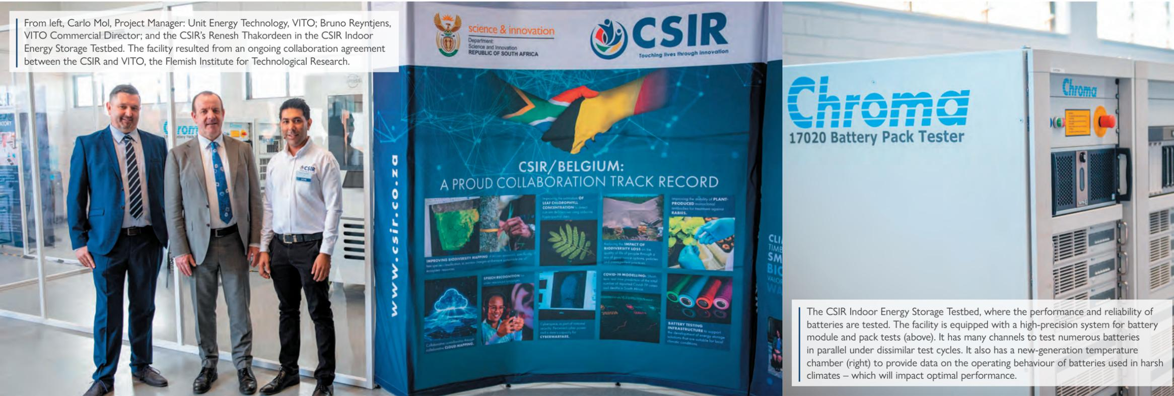
The CSIR Indoor Energy Storage Testbed, where the performance and reliability of batteries are tested. The facility is equipped with a high-precision system for battery module and pack tests (above). It has many channels to test numerous batteries in parallel under dissimilar test cycles. It also has a new-generation temperature chamber (right) to provide data on the operating behaviour of batteries used in harsh climates – which will impact optimal performance.
