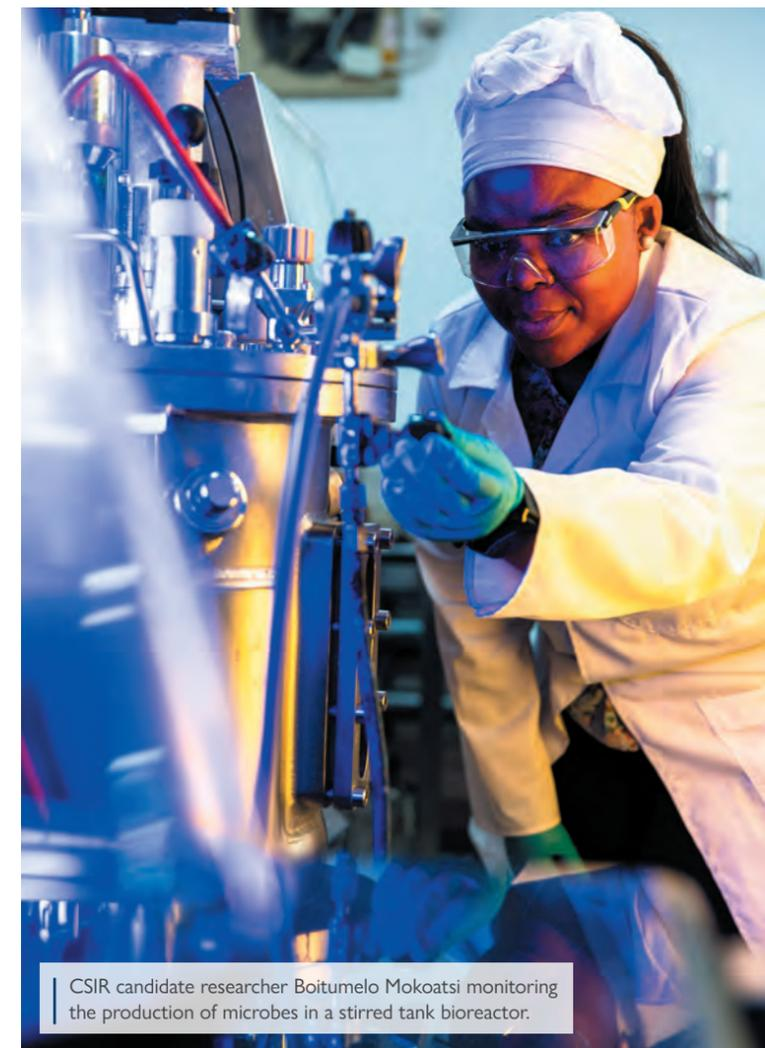
CSIR candidate researcher Boitumelo Mokoatsi monitoring the production of microbes in a stirred tank bioreactor.
