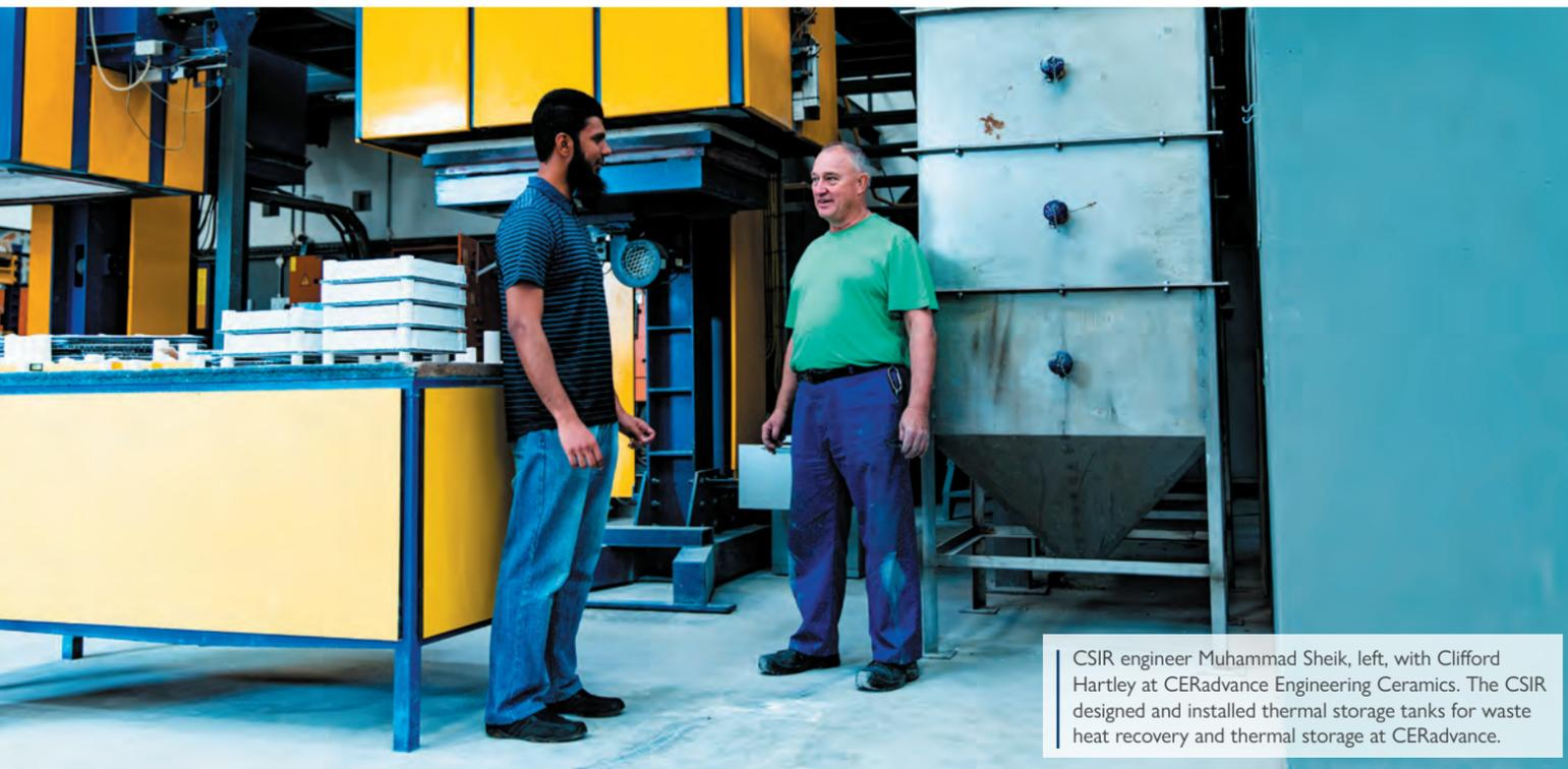
CSIR engineer Muhammad Sheik, left, with Clifford Hartley at CERadvance Engineering Ceramics. The CSIR designed and installed thermal storage tanks for waste heat recovery and thermal storage at CERadvance.
