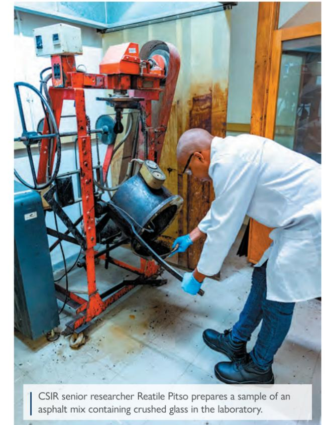
CSIR senior researcher Reatile Pitso prepares a sample of an asphalt mix containing crushed glass in the laboratory.
