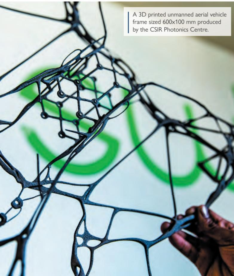
A 3D printed unmanned aerial vehicle frame sized 600x100 mm produced by the CSIR Photonics Centre.
