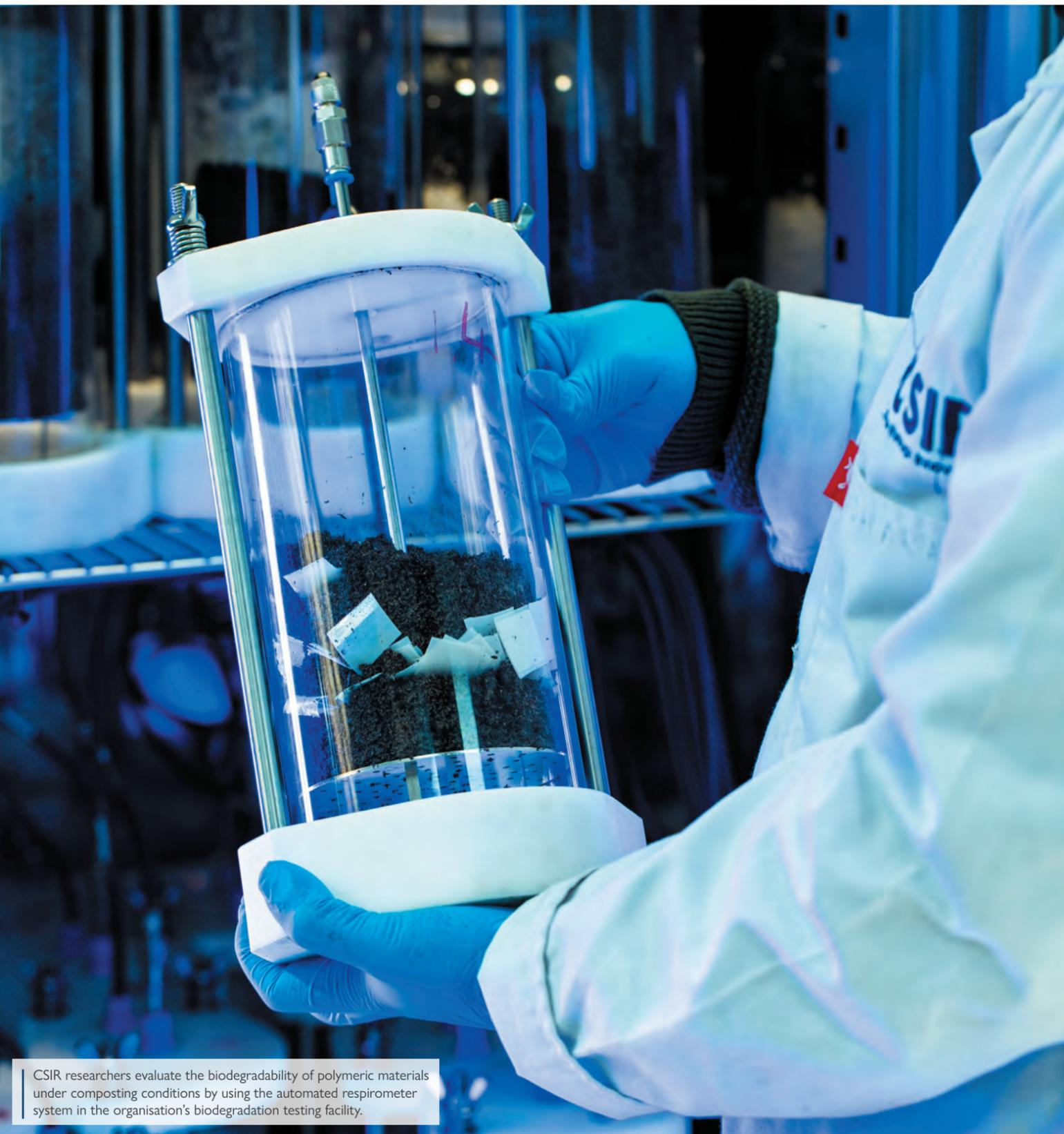
CSIR researchers evaluate the biodegradability of polymeric materials under composting conditions by using the automated respirometer system in the organisation's biodegradation testing facility.
