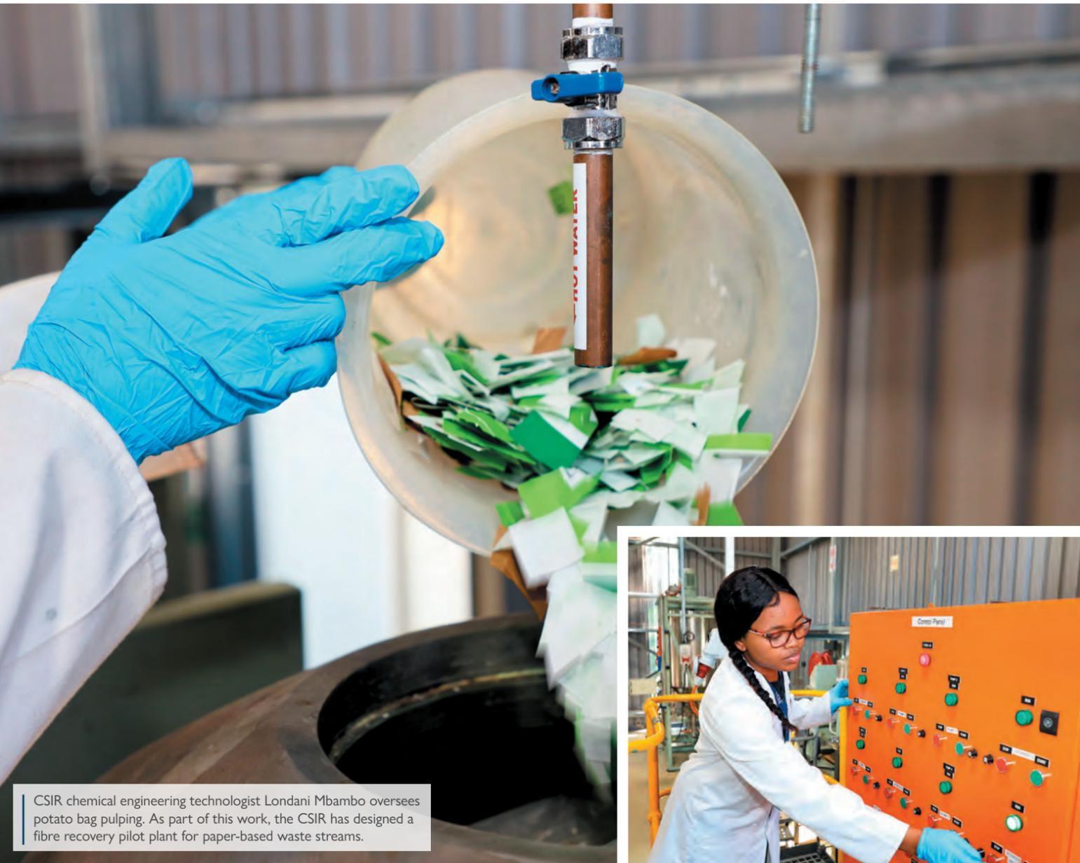
CSIR chemical engineering technologist Londani Mbambo oversees potato bag pulping. As part of this work, the CSIR has designed a fibre recovery pilot plant for paper-based waste streams.
