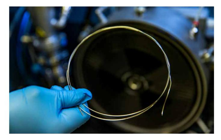
The CSIR Powder Atomisation has a modern, compact ultrasonic atomiser designed to create spherical powders from metal wires and rods. This facility aims to replace imported spherical metal powders, which currently face issues with high costs and long lead times.
