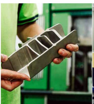
Investment casting is an industrial manufacturing process that has a very long history, dating back 4000 years. Since then, significant advances have been achieved in wax and shell materials and vacuum casting technologies to enable intricate and high-integrity castings to be produced for the most demanding of applications.
