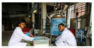
CSIR chemical engineering intern, Zandile Mabasa, and chemical engineering graduate trainee, Simphiwe Ncwane, collect a slurry product from a reactor.
