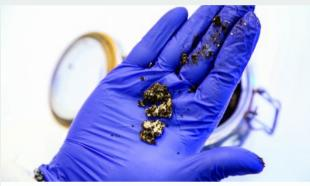
A researcher demonstrates the test kit before (top) and after 60 days (above) of disintegration under controlled composting conditions, as per standards set by the American Society for Testing and Materials.
