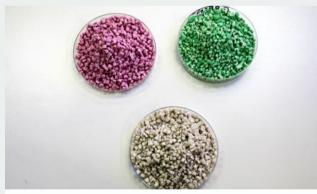
CSIR developed biopolymers and biobased additives pellets used to produce biodegradable test kit cassettes and surgical aprons, which are an environmentally friendly alternative to current petroleum-based plastics.
