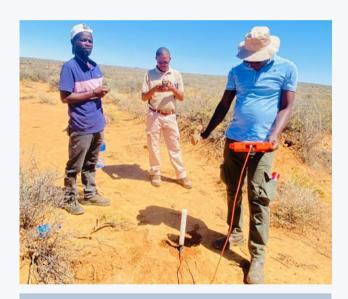
CSIR researchers are using modern hydrogeophysical methods to map aquifer systems below the ground in De Aar, Northern Cape. The results of such a survey allow municipal managers to strategically manage groundwater by scheduling and switching borehole pumping in a way that will not deplete aquifers. At the same time, the water quality data these surveys provide can inform water treatment measures that will ensure sustainable, clean and safe drinking water for their communities.
