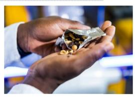
The biodegradable food packaging film produced at the CSIR pilot facility in Pretoria. The packaging blocks oxygen, thereby preventing spoilage and extending shelf-life. The polymers are also stable at high temperatures and have improved composting properties.
