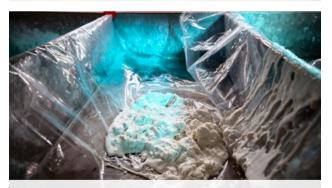
Metal-organic framework cakes are collected after mechanical dewatering using a pilot-scale filter press.
