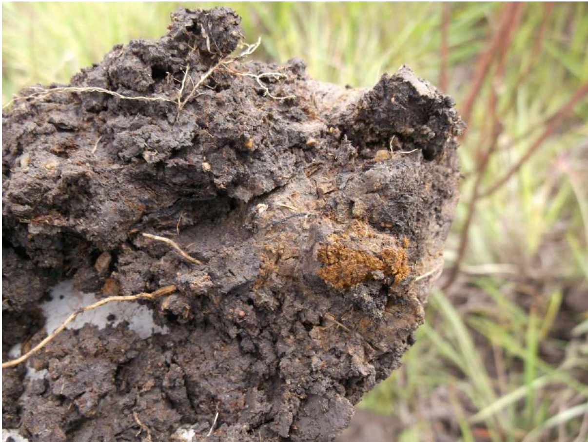
Figure 5.2: Soils of the stream bed indicating a prominent grey matrix with few mottles and thus the permanent zone.
