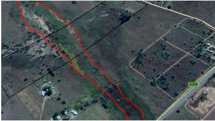
Figure 47: The highlighted area showing the artificial drainage line draining the valley bottom from water entering the seep
