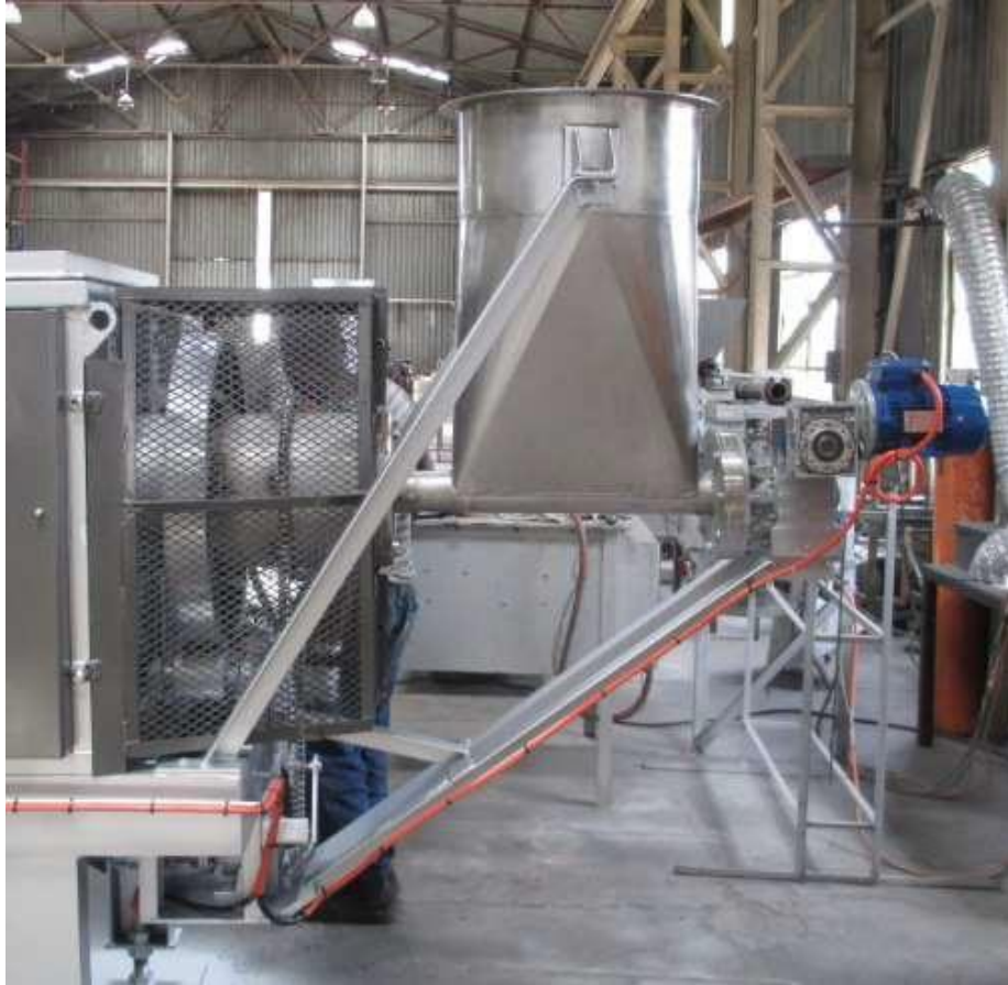
Figure 3 - Feed Screw and Surge Hopper on a Specialized Feeding System on a small rotary kiln.
