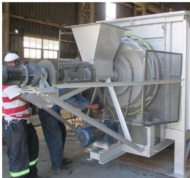
Figure 2 - Drive Motor, Chain and Sprocket on a Rotary Kiln.
