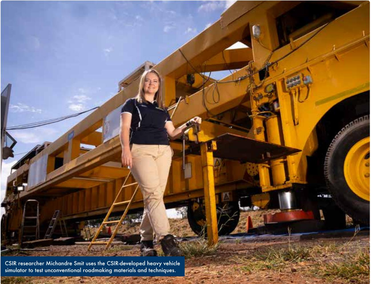
**The CSIR has conducted the first test of a new geogrid design intended to strengthen and stabilise material used in road construction. The test was done for an international client, using the CSIR-developed heavy vehicle simulator (HVS).**
