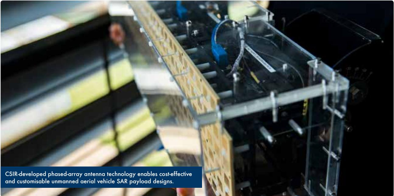
CSIR-developed phased-array antenna technology enables cost-effective and customisable unmanned aerial vehicle SAR payload designs.
