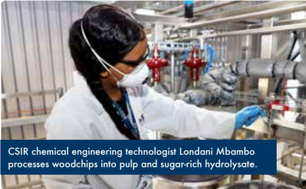
CSIR chemical engineering technologist Londani Mbambo processes woodchips into pulp and sugar-rich hydrolysate.
