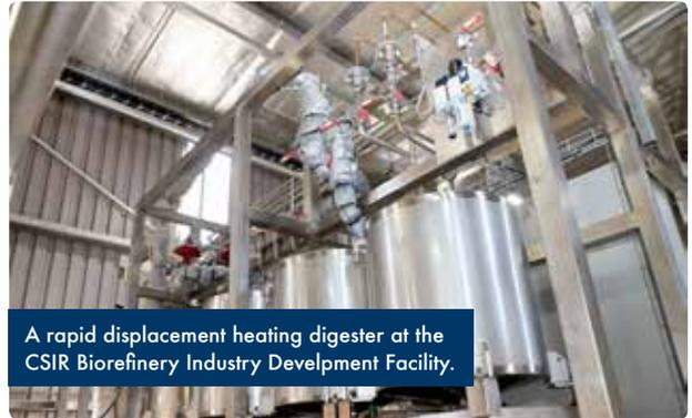
A rapid displacement heating digester at the CSIR Biorefinery Industry Development Facility.
