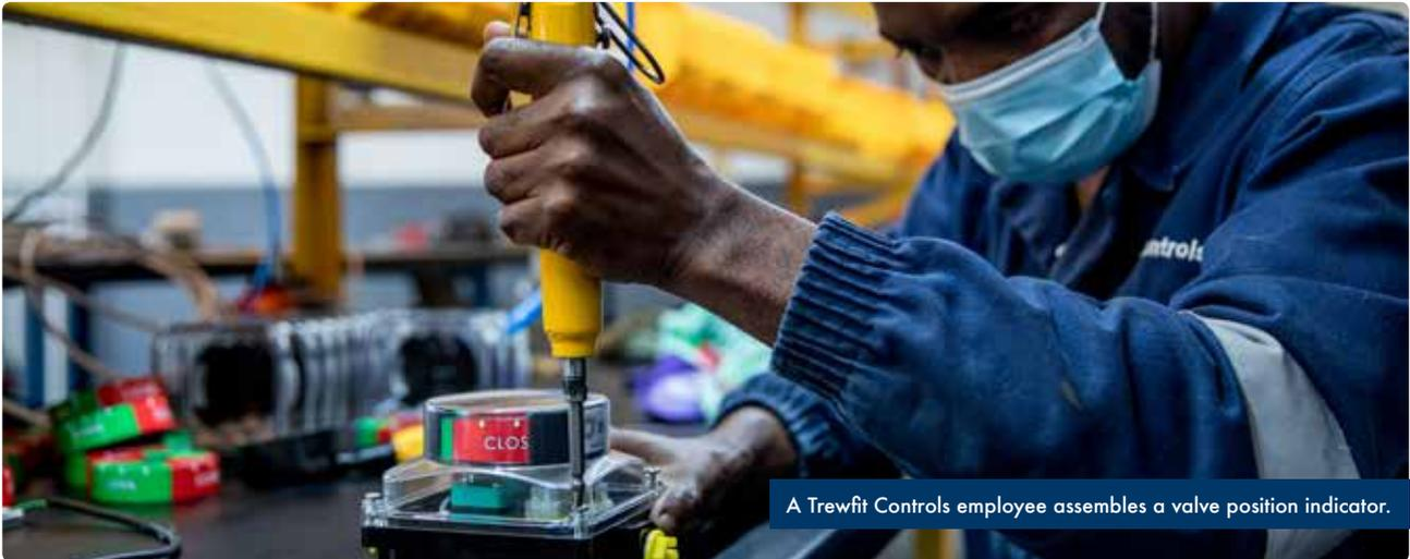
A Trewfit Controls employee assembles a valve position indicator.
