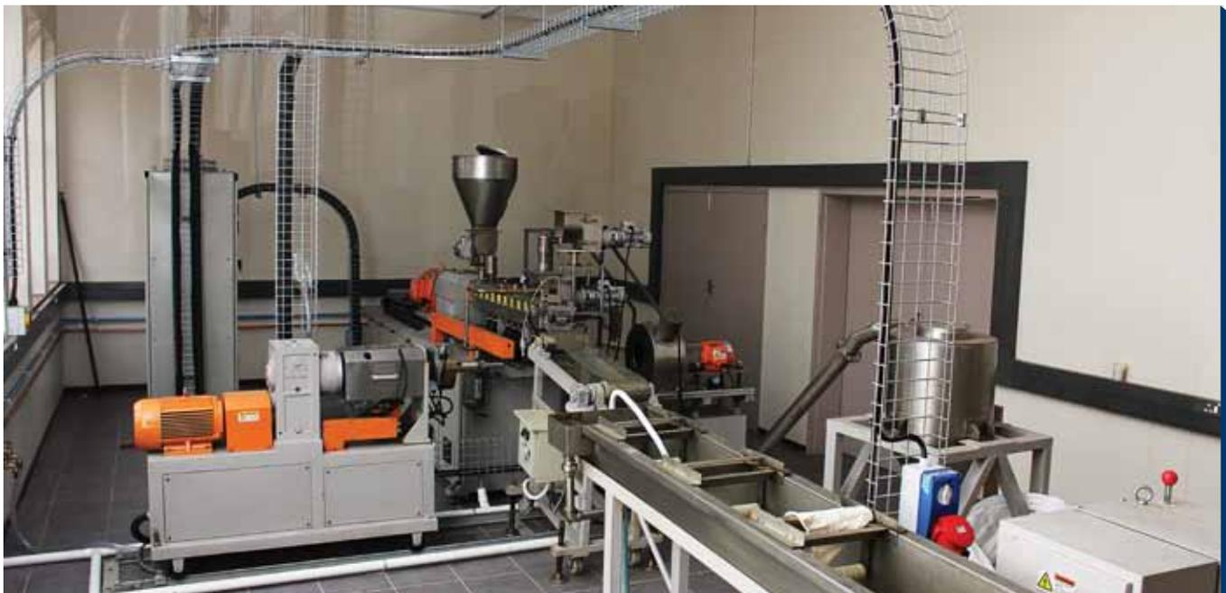
The newly-acquired, industry-scale extruder at the National Centre for Nano-Structured Materials is a machine which is normally used for melting a plastic polymer and then converting it to a certain shape through a process called extrusion. The extruder can be used to mix the polymer with additives or nanostructured materials to prepare a polymer nanocomposite in order to enhance the properties of the polymer such as fire retardance performance.
