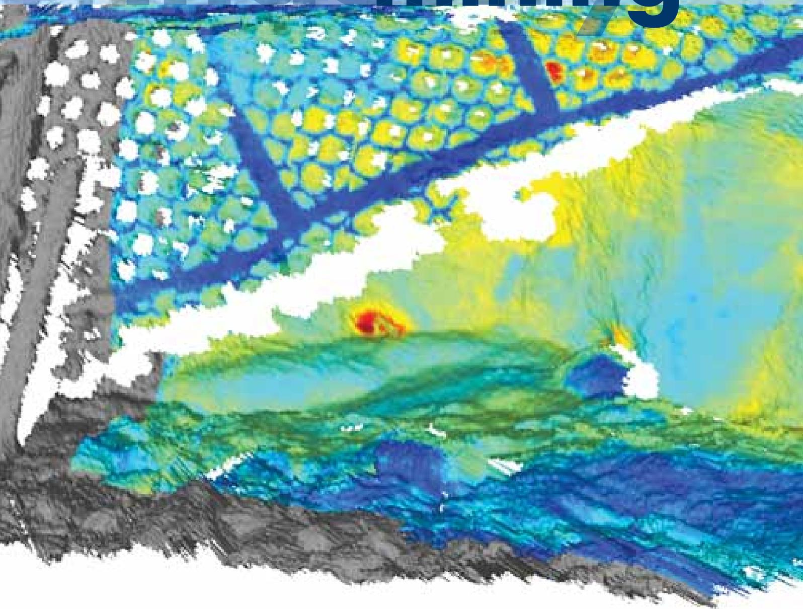
This visualisation of a mine stope acquired with a CSIR multi-sensor 3D scanner shows a portion of a 3D model of a platinum mine stope face, coloured by rock temperature. These visualisations are helpful in determining areas where a unique combination of temperature and structure indicates an area of potential rock fall risk where remedial action is required to make the area safe.
