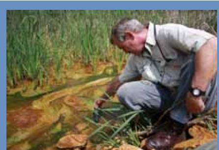
CSIR geohydrologist Phil Hobbs measuring the pH of acidic mine water decanting from abandoned mines in the Western Basin.
