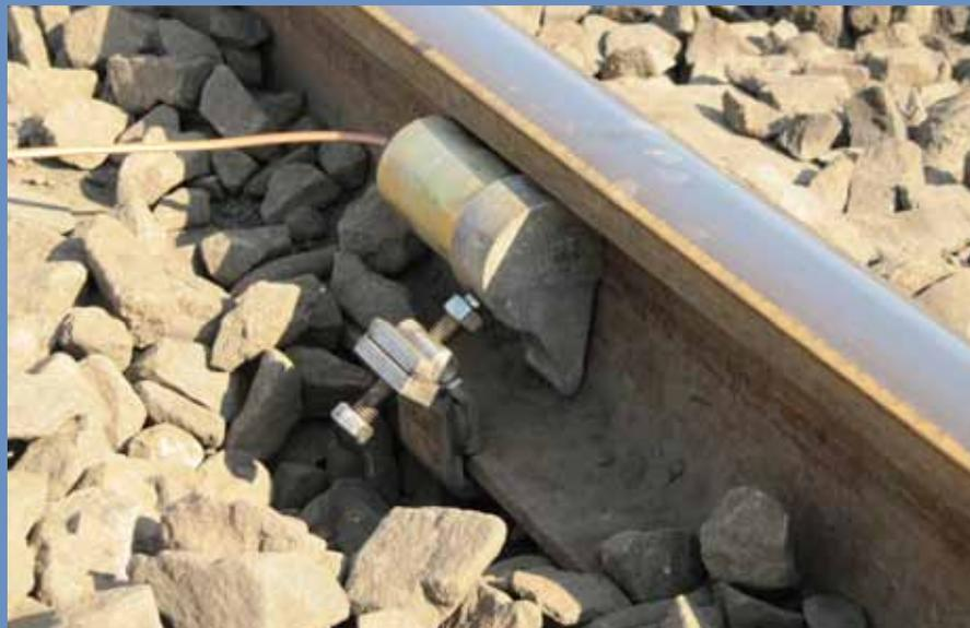
Custom ultrasound transducer for rail break monitoring, attached to the Sishen-Saldanha heavy freight railway line.
