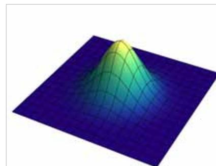
Image of a 'nice' laser beam, i.e. a laser beam of good quality and high energy: a Gaussian-shaped intensity profile.
