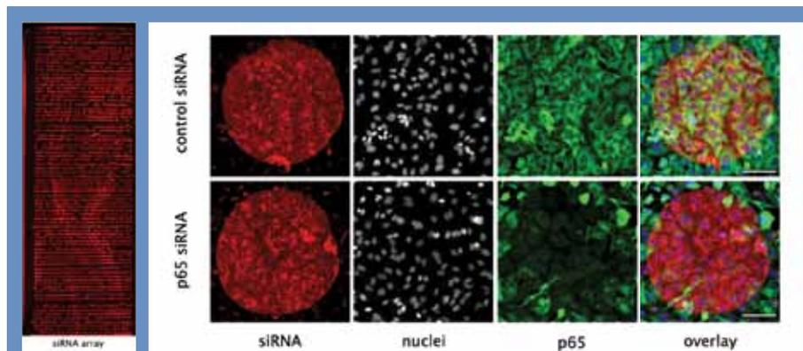
(Left) Each red spot on this array – a single printed experiment – is equal to a test tube or beaker in the laboratory. With high throughput biology the number of experiments can be increased dramatically and the time of execution decreased. On the right, the top row shows a controlled experiment where all the genes are active. The bottom row shows the effect of one gene being silenced in an experiment.
