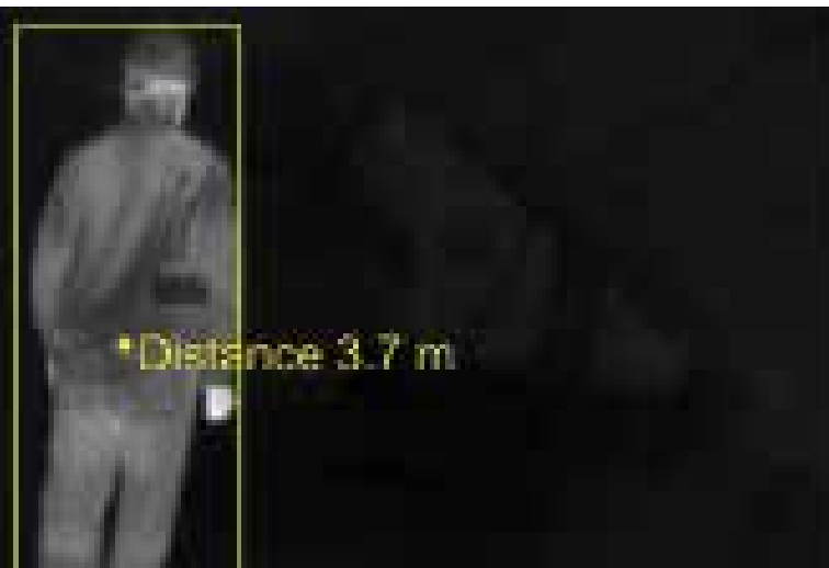
CSIR researcher John Dickens with a thermal imaging system developed to prevent collisions between rail-bound mine vehicles and mine workers. A grey-scale thermal image (right) shows a pedestrian at a distance of 3.7 m.
