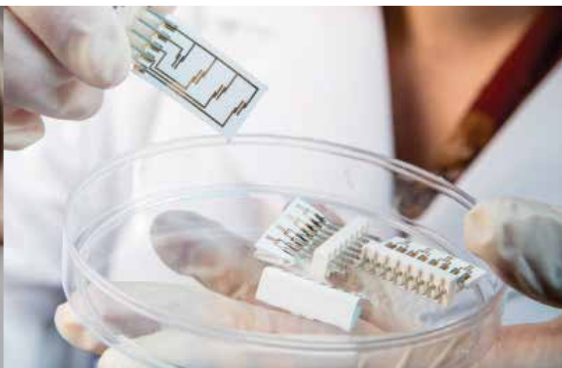
An example of printed electronic circuits used for environmental diagnostics.
