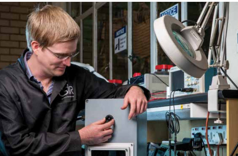
CSIR researcher John Dickens with a thermal imaging system developed to prevent collisions between rail-bound mine vehicles and mine workers. A grey-scale thermal image (right) shows a pedestrian at a distance of 3.7 m.
