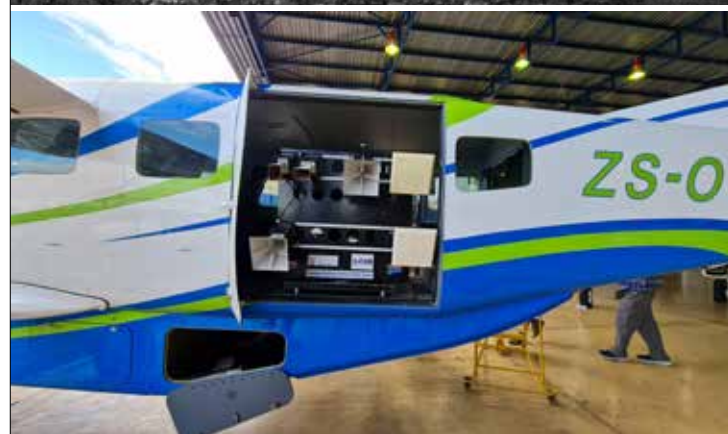
Clockwise from top: Funded by the Department of Science and Innovation, this CSIR-developed airborne synthetic aperture radar (SAR) facility is the first of its kind in South Africa. The first baseline technology demonstrator for a phased array satellite SAR payload. The airborne SAR facility installed onboard a Cessna 208 airplane during a recent multi-sensor campaign flight. A high-resolution SAR image captured over Rayton, near Pretoria, using the CSIR-developed SAR technology.
