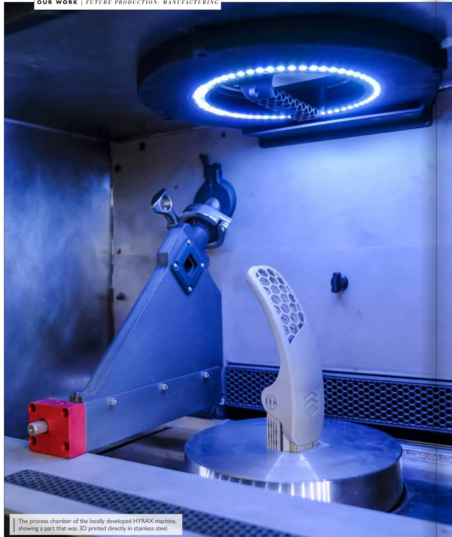
The process chamber of the HYRAX machine with a 3D-printed part.
