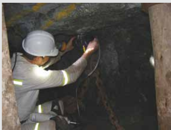
A CSIR engineer installs a wireless sensor in a platinum mine stope.
