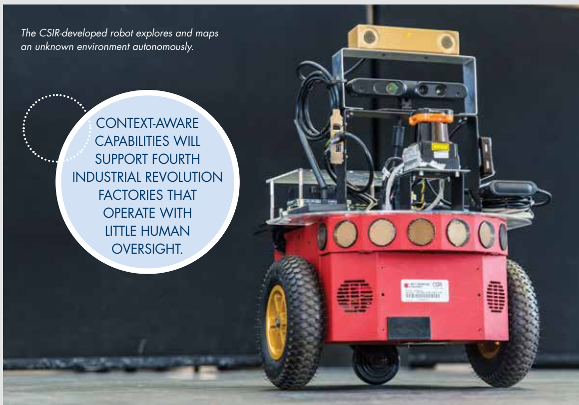
Key features of the robot include a stereo-vision camera (the gold coloured sensor at the top) for 3D imaging, and a low-power, mobile graphics processing unit (mounted at the back of the robot) for real-time image analysis.
