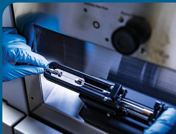
Dr Previn Naicker loads calibrant solution onto a syringe pump of the mass spectrometer and (below) adjusts the gas control on the tims cell of the mass spectrometer.
