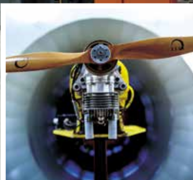
Above: The engine reliability test rig was developed to support the development of unmanned aerial vehicles (UAVs). The rig has been used to test the functioning of the new UAV engine systems and to optimise the engine cowling ducting in the wind tunnel. During tests, many engine and environmental parameters are logged and summarised data or emergency shut-down data are transmitted to the test personnel involved.
