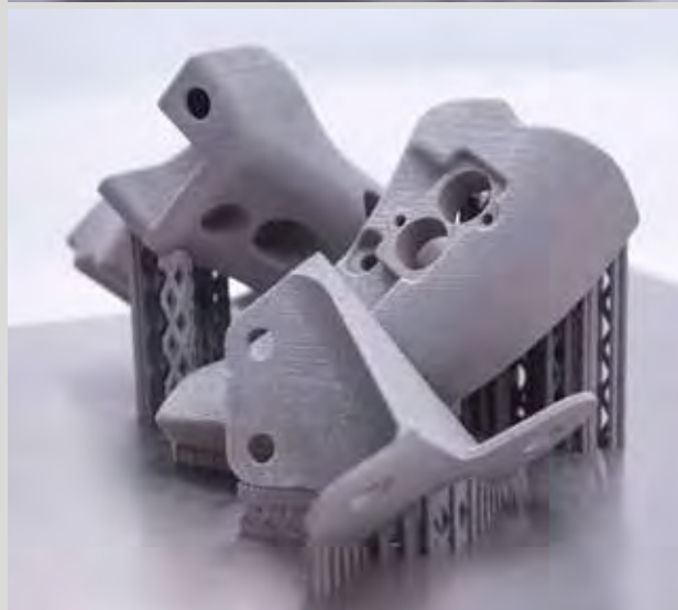
The Aeroswift team produced two different flight grips (the condition lever grip and throttle grip) for the South African developed AHRAC aircraft. The titanium metal part on the far right of the top image is a fuel pylon bracket developed for a commercial aircraft. The bottom image shows the parts from a different angle.
