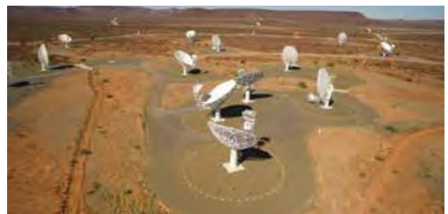
An aerial view of the MeerKAT core at the SKA project's Losberg site in the Karoo, in the Northern Cape. The MeerKAT radio telescope array will consist of 64 antennas which will be integrated into the first phase of the SKA project. Image courtesy SKA South Africa
