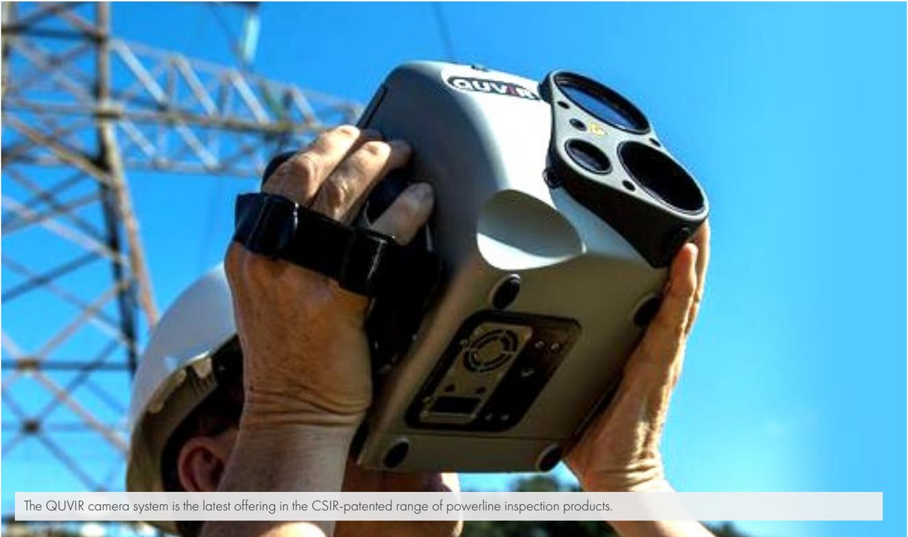
The QUVIR camera system is the latest offering in the CSIR-patented range of powerline inspection products.
