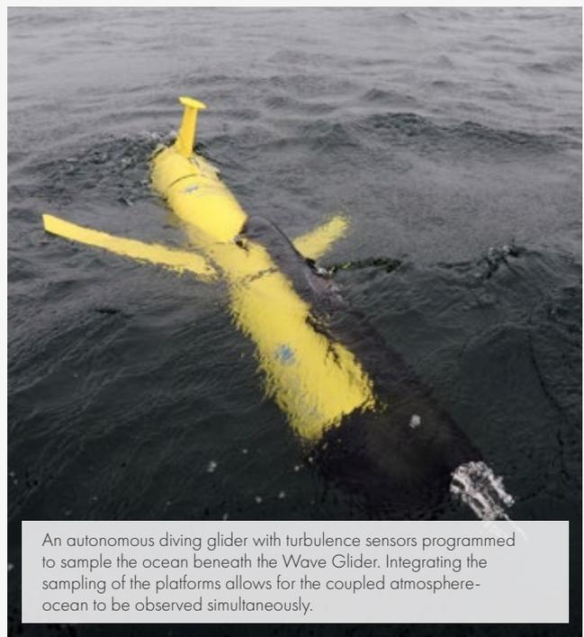
An autonomous diving glider with turbulence sensors programmed to sample the ocean beneath the Wave Glider. Integrating the sampling of the platforms allows for the coupled atmosphere-ocean to be observed simultaneously.
