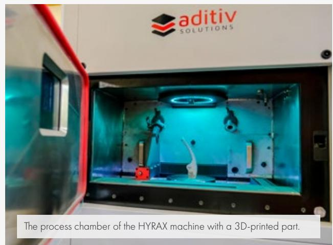
The process chamber of the HYRAX machine with a 3D-printed part.
