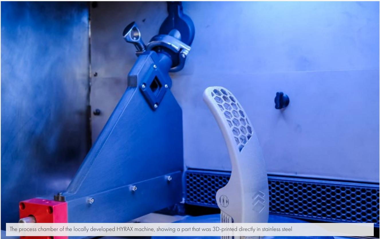
The process chamber of the locally developed HYRAX machine, showing a part that was 3D-printed directly in stainless steel
