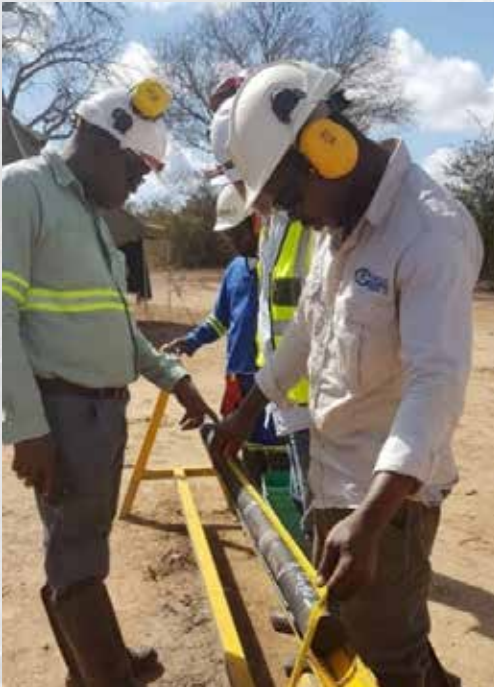
Geotechnical core logging
