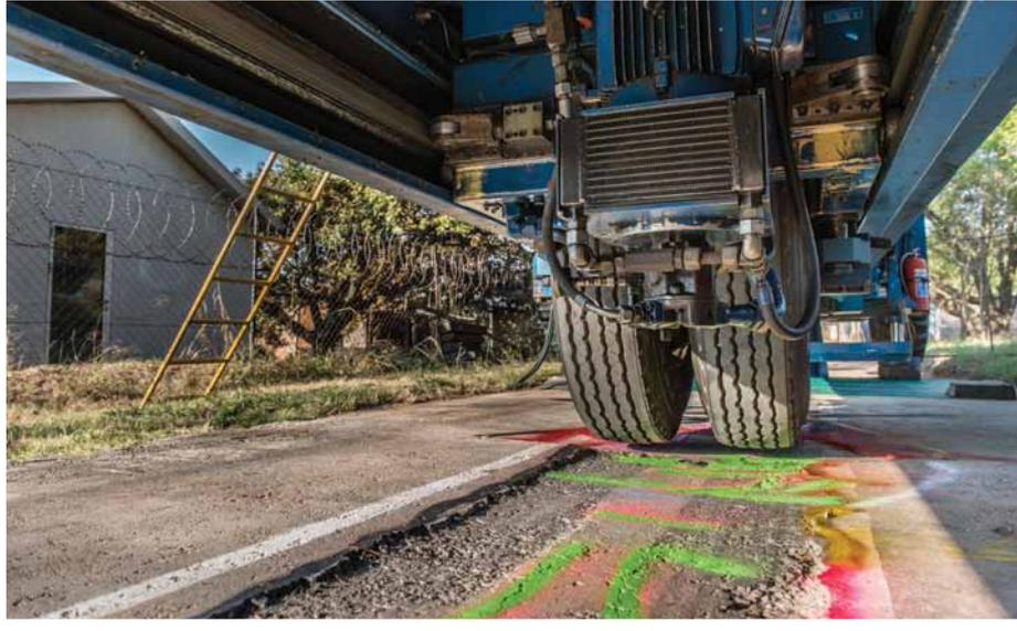
A road is designed to last between 20 and 30 years if constructed and maintained correctly. This implies that when a new material or design is developed, a trial section needs to be built to evaluate how it responds to being subjected to traffic for many years – a costly and time-consuming approach. The CSIR's heavy vehicle simulator is a mobile laboratory used by decision-makers and road builders to apply and monitor the effect of 20 years of traffic to a road section in just three months.
