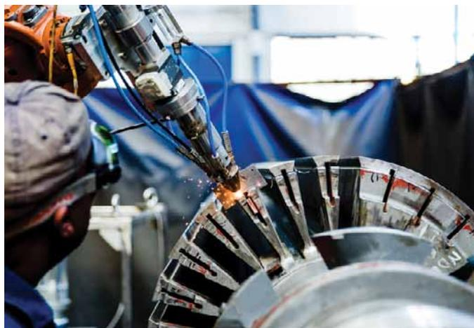
◀ Left: The CSIR’s 3D laser-cutting capability offers a cost-effective solution for manufacturing of formed components. ▲ Above: The CSIR has built a strong competence in laser-based refurbishment based on laser cladding technology. This technology is best suited for the repair of large and high-value components, such as generator rotors.
