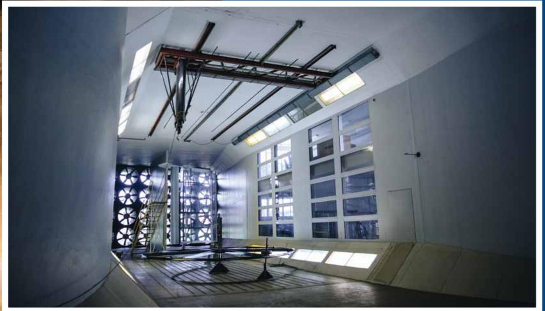
The CSIR's suite of wind tunnels provides a specialised research and experimental environment that supports the aerodynamic design efforts of the South African aeronautics industry. Testing in a wind tunnel simulates the flow environment encountered by an aircraft during flight.
