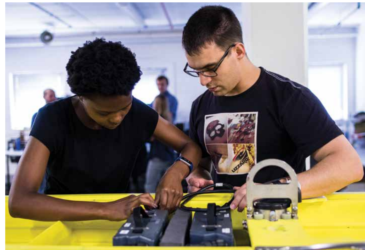
Above: Zimkhitha Mbekeni (left) from the Cape Peninsula University of Technology and Ryno Els from STS checking the underwater connector on a wave glider's electronic enclosures.
