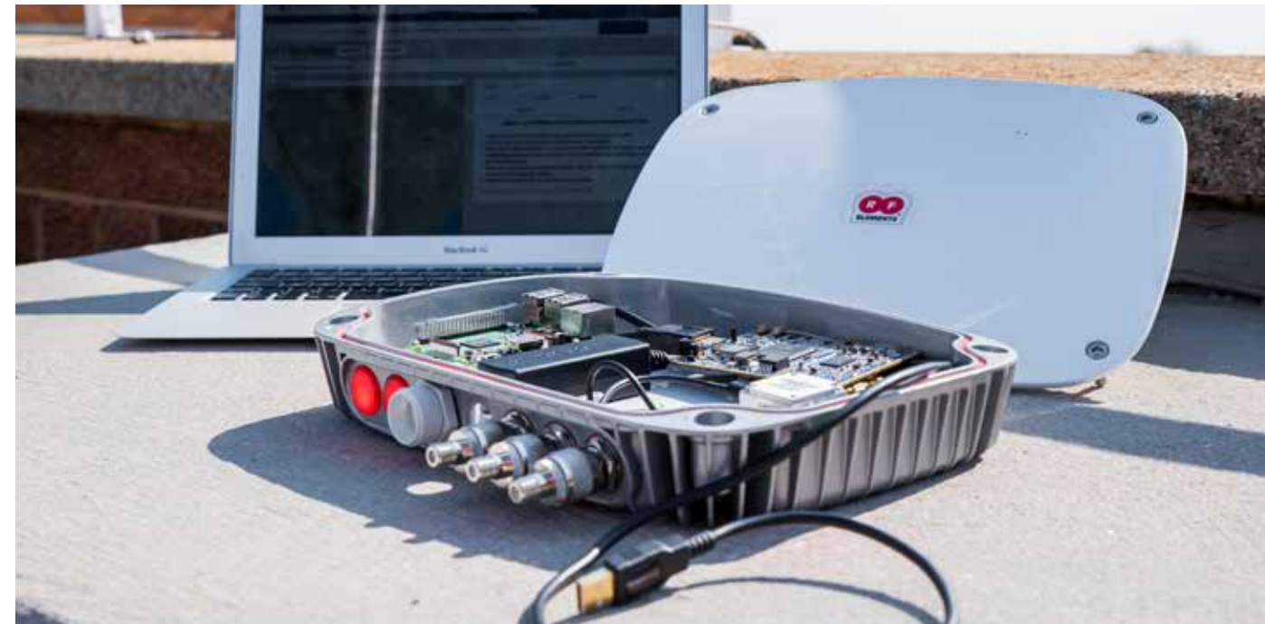
Above: A prototype of the CSIR-developed low-cost spectrum monitoring device.
