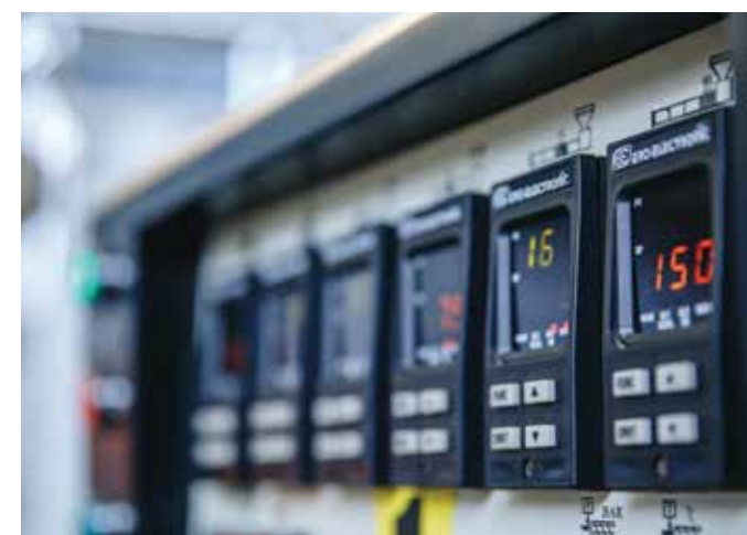
Above: The control panel of a five-layer film blower inside the NIDF.
