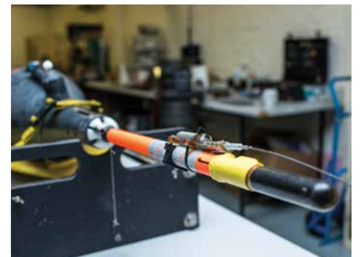
Above: The antenna of a Seaglider, an autonomous underwater vehicle, is inspected before deployment.
