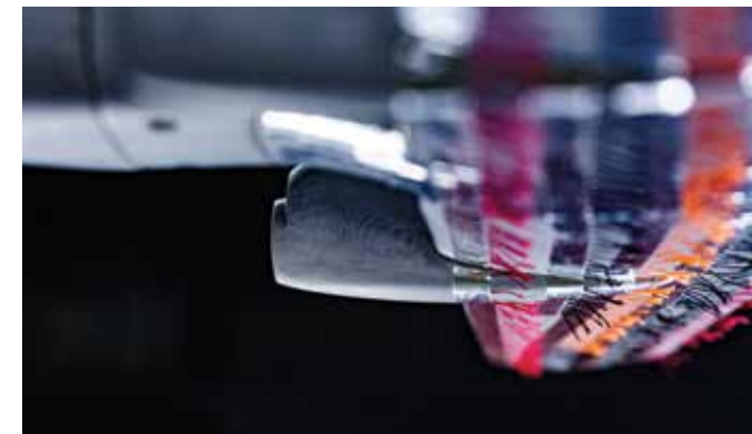
Above: The CSIR's first all 3D-printed polymer aircraft model set up for testing in the low-speed wind tunnel.
