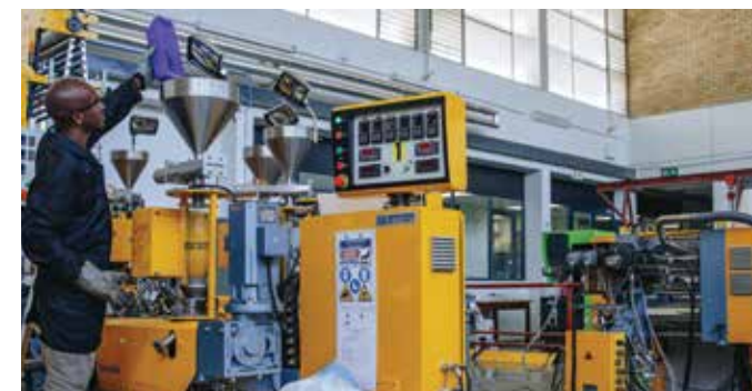
Above: Feeding of the coextrusion film blower with polymer pellets to make a high-barrier packaging film.
