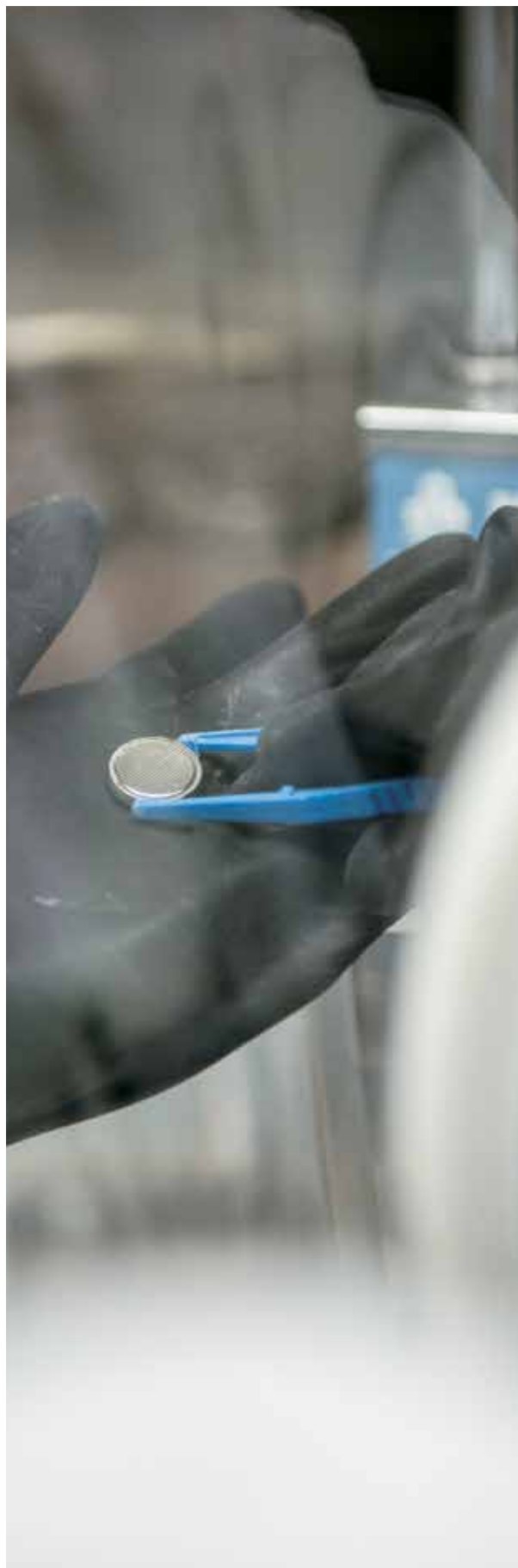
Button cell lithium-ion battery produced at the CSIR.
