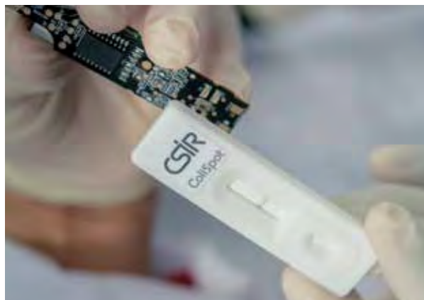
The low-cost E. coli detection device, ColiSpot.
