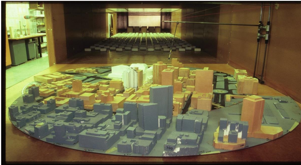
Figure 2: Typical model of the urban environment and the flow-processing devices
