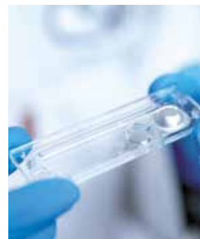
A microfluidic cartridge device for blood cell counting applications.
