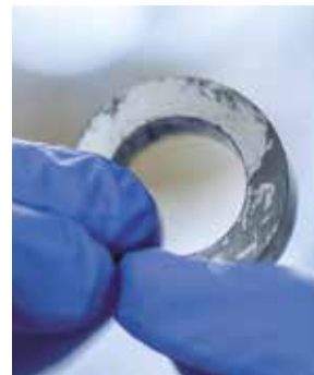
A compacted automobile valve seat insert produced using titanium powder.
