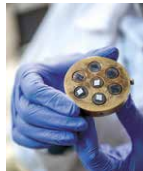
A sample stage with various samples prior to examination using scanning electron microscopy. Using this instrumentation, seemingly uninformative details to the naked eyes are translated into valuable information about the nanostructure of materials.
