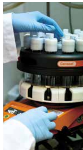
Testing catalyst activity on multiple substrates using the Carousel reactor.
