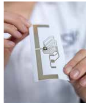
An example of a printed electronic device containing a printed antenna for potential integration with paper-based microfluidic devices.
