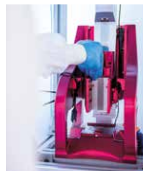
A high-throughput microarray printer is used to screen compounds.
