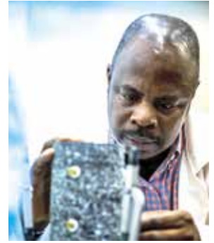
Dr Anochie-Boateng tests the stiffness, rutting and cracking resistance of asphalt.
