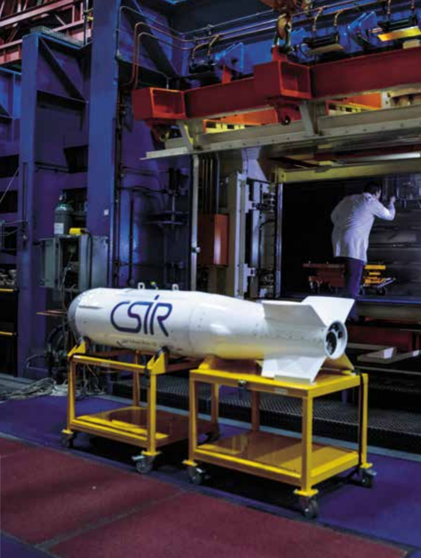
The radar and electronic warfare pod being prepared for tests in the transonic wind tunnel at the CSIR.
