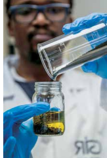
Above and below: CSIR researchers doing experiments on the use of nanocomposites as a low-cost adsorbent to remove chromium (VI) from wastewater.
