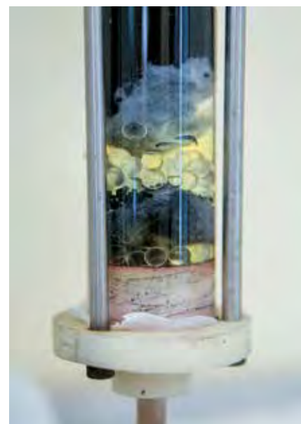
Above and below: CSIR researchers doing experiments on the use of nanocomposites as a low-cost adsorbent to remove chromium (VI) from wastewater.
