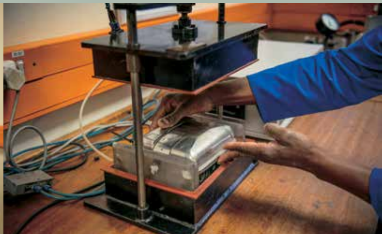
A self-contained self-rescuer being leak tested on the electronic leak detector.
