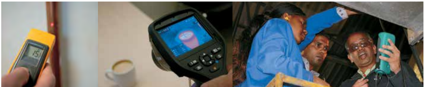
(From left) An infra-red thermometer; thermal imaging camera for steam systems; and steam system expert level training.
