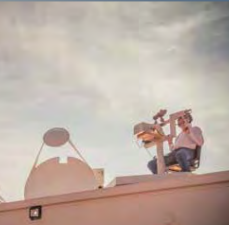
Positioned at an elevated level, the optical target designator has a broader field of view to detect a target – on the sea or in the air.
