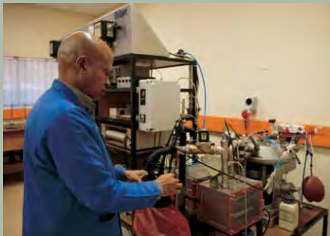
Richard Rapoo undertakes functional tests on the breathing simulator of the self-contained self-rescuer.
