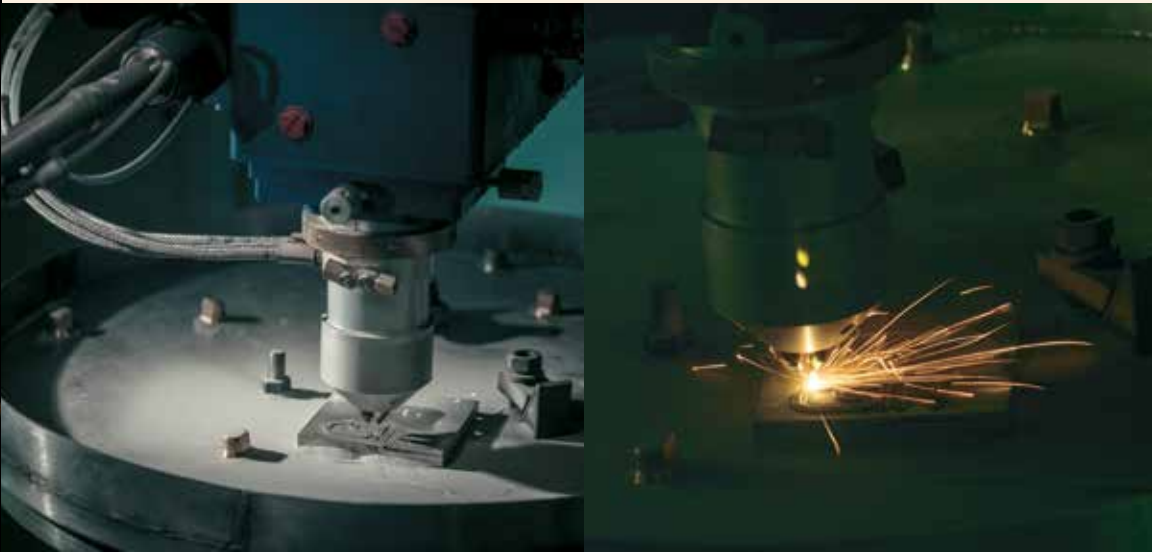
The technology used in the laser-engineered net-shaping system (LENS) involves a high-power laser (500 W to 4 kW) to fuse powdered metals into fully dense, three-dimensional (3D) structures. The LENS 3D system uses the geometric information contained in a computer-aided design solid model to automatically drive the LENS process as it builds up a component, layer by layer (as shown in the pictures).
