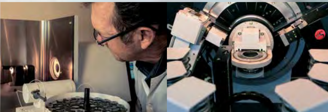
Atomic absorption spectroscopy is shown. This is an instrument used for the analysis of elements in a given liquid sample using either a flame or graphite furnace.
