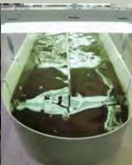
Laboratory-scale algal raceway pond.
