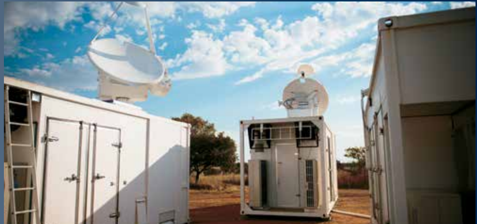
The Fynmeet II and Taba radars in this mobile facility form a radio frequency signal measurement system that tracks and measures targets. Measurements enable the operator to identify the specific target type.
