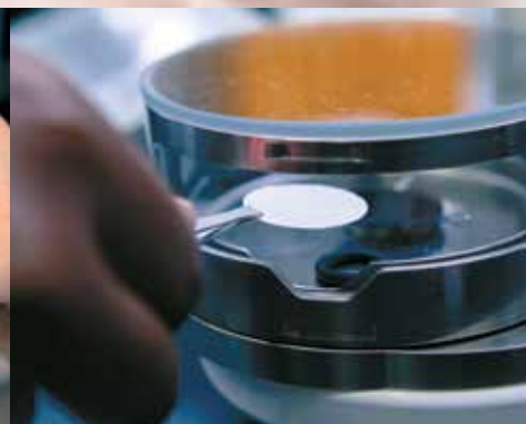
Gravimetry or weighing, a technique used for weighing filter papers either with dust or without dust.
