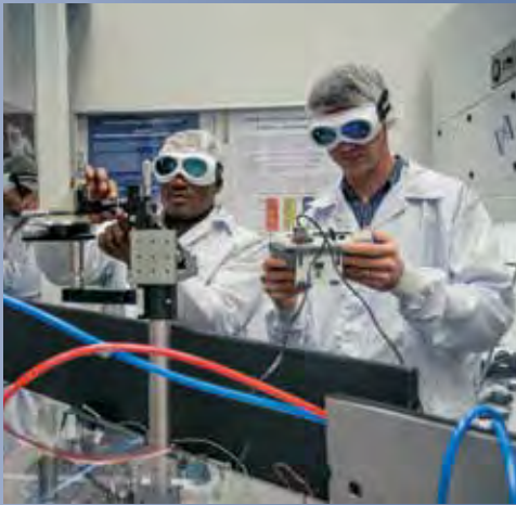
Ramokolo aligns the camera for beam shape measurement and Marius Vermeulen from Aerosud observes the power meter display.
