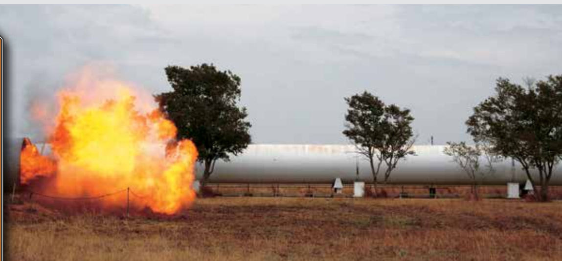
The 200 m explosion gallery is used for research on novel methods to prevent fires and explosions.
