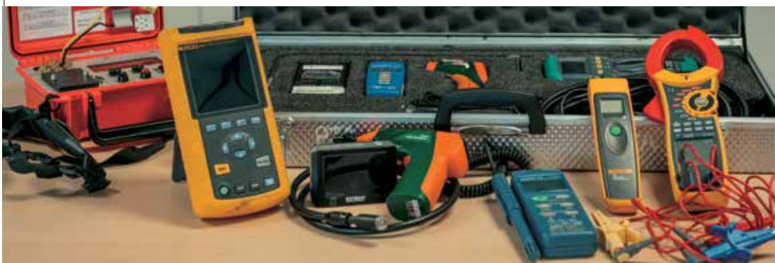
(From left) A flow kinetics FKT electronic manometer for fan systems (back); a power meter for measuring KW, Amps and Volts; an infra-red thermometer; a humidity/temperature meter for fan systems; another infra-red thermometer and a current clamp (also seen on page 38).
