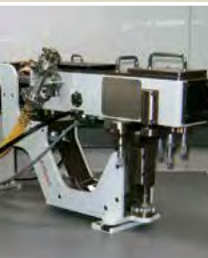
Small-angle x-ray scattering is a non-destructive method for investigating nano-structures from less than a 1 nm up to 200 nm in size.
