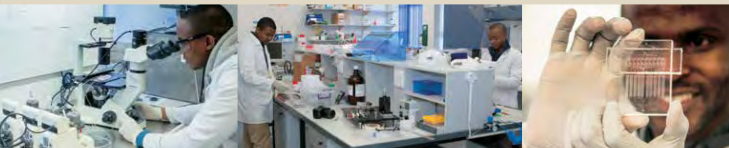
(From left) Pressure pumps for controlling fluid flow in microfluidic devices; development of cartridge-based microfluidic devices; microscopes available in the laboratory; the microfluidic testing facility; and an example of a microfluidic device manufactured in the facility.
