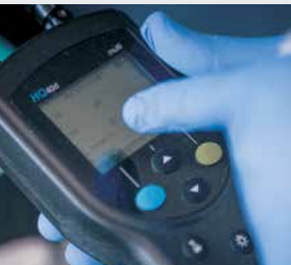
The acidity levels, electrical conductivity and total number of dissolved solids are measured inside the aeration chambers of the simulated wastewater treatment plant after samples had been taken.
