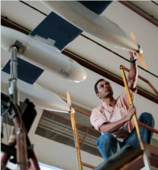
An aeronautical engineer doing a final inspection on a wind tunnel model.
