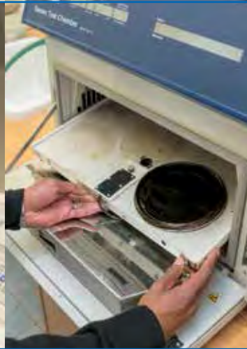
A Q-Sun Xenon test chamber used for ultraviolet testing of, for example, paint.
