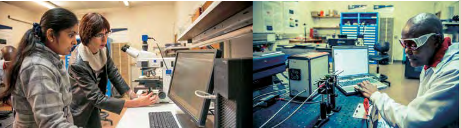
State-of-the-art equipment in the advanced photonics laboratory includes an inverted microscope for inspection of optical surfaces, here used by Ann Singh and Dr Aletta Karsten (and seen up close on page 10). CSIR technician Bafana Moya is seen with a fibre-based spectrometer covering a wavelength range from 1 100 nm to 2 400 nm.
