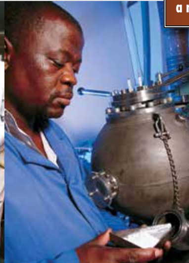
Industrial dust explosion test in the 20 litre explosion vessel.
