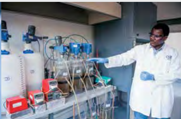
Senior researcher Dr John Zvimba showing a simulated wastewater treatment plant, the only of its kind in the Southern Hemisphere, where wastewater from Daspoort treatment plant is used for contamination with different nanomaterials in a continuous process.
