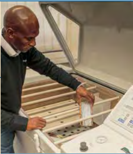
Rust resistance is tested inside a Q-Fog salt spray chamber.
