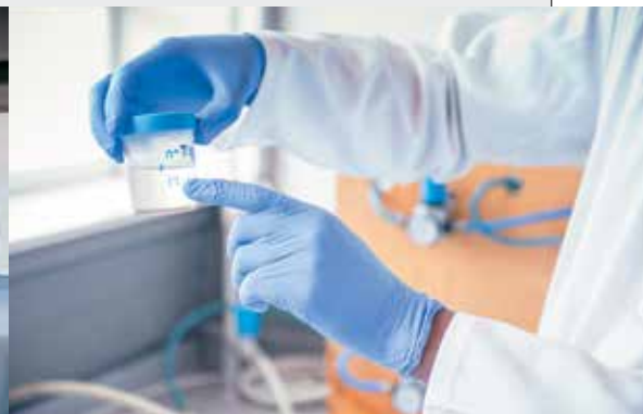
A sample of water and sludge from the aeration chambers of the simulated wastewater treatment plant. Samples are taken three times a week and then twice on those days at exactly the same time, to analyse and compare the microorganisms therein.
