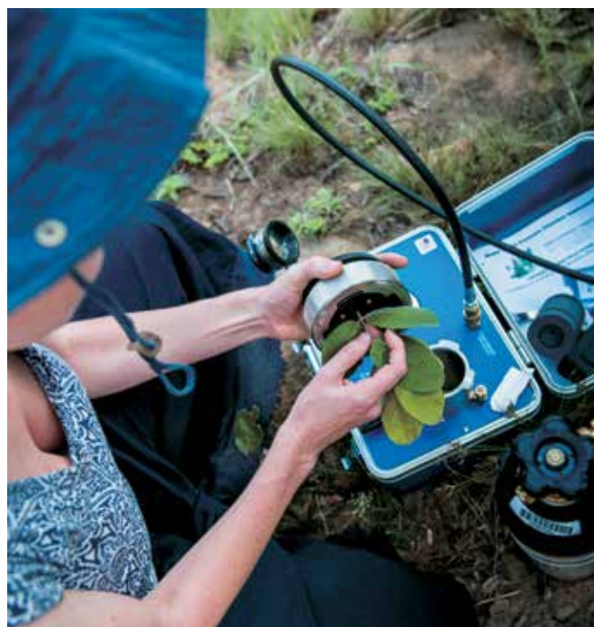
Above and background: Dr Sally Archibald tests the water potential of savannah trees using a Scholander Pressure Device. This is a simple, reliable method for assessing the water stress of a plant.
