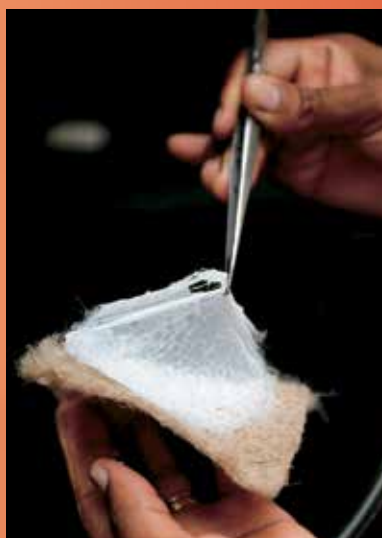
Left: Nanofibrous material (web) of which the individual fibres have a diameter in the nano range. These fibres were electrospun directly onto a nonwoven mat for filtration purposes.
