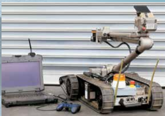
The PackBot 510 is a robotic platform equipped with a laser scanner and on-board computer which is used for safety inspection of mine stopes immediately after blasting. It is also used for urban search and rescue projects. The Packbot 510 is controlled from an operator console which is a laptop with a joystick.
