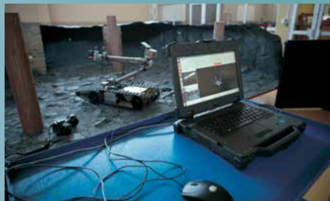
The PackBot 510 inside an artificial mine stope with the operator console showing the user interface. This consists of video streams from the PackBot 510 and the map of the environment. These robots can operate autonomously, semi-autonomously (by giving it goals) and manually (using a joystick).
