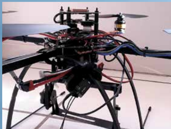
A low-cost, unmanned aerial vehicle for ecological visual surveillance and decision support.
