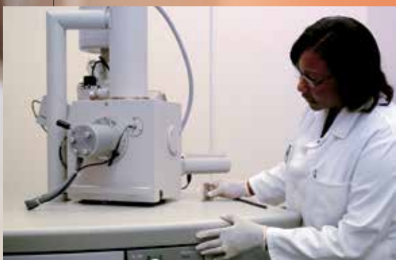
Above: Dr Valencia Jacobs uses an Environmental Scanning Electron Microscope, one of the tools used to determine the characteristics of electrospun nanofibres.
