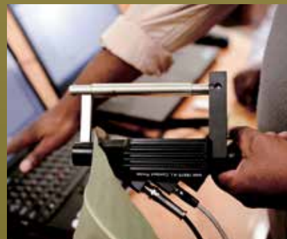
An analytical spectral device used to measure leaf reflectance.
