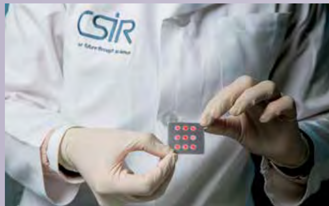
A wax-printed paper-based microfluidic device. Reactions implemented on the device result in a colour change.
