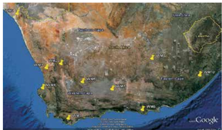
Figure 2: Location of measurement sites within the project domain. The project required three years of measurement data from the ten measurement sites for the verification. Each site consisted of a 60 m mast with anemometry at 62 m, 60 m, 20 m and 10 m as well as other meteorological sensors. The data from the sites were sent to the CSIR where it was quality controlled and made available on the WASA web site.
