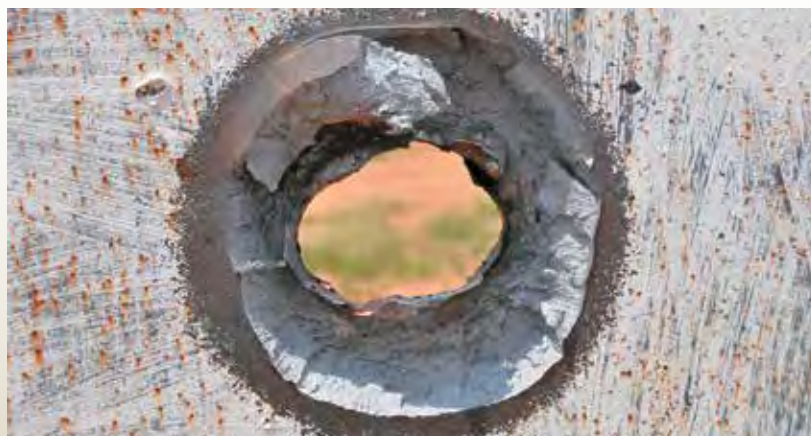
Typical damage or penetration caused due to an improvised explosive device projectile on an unprotected target.
