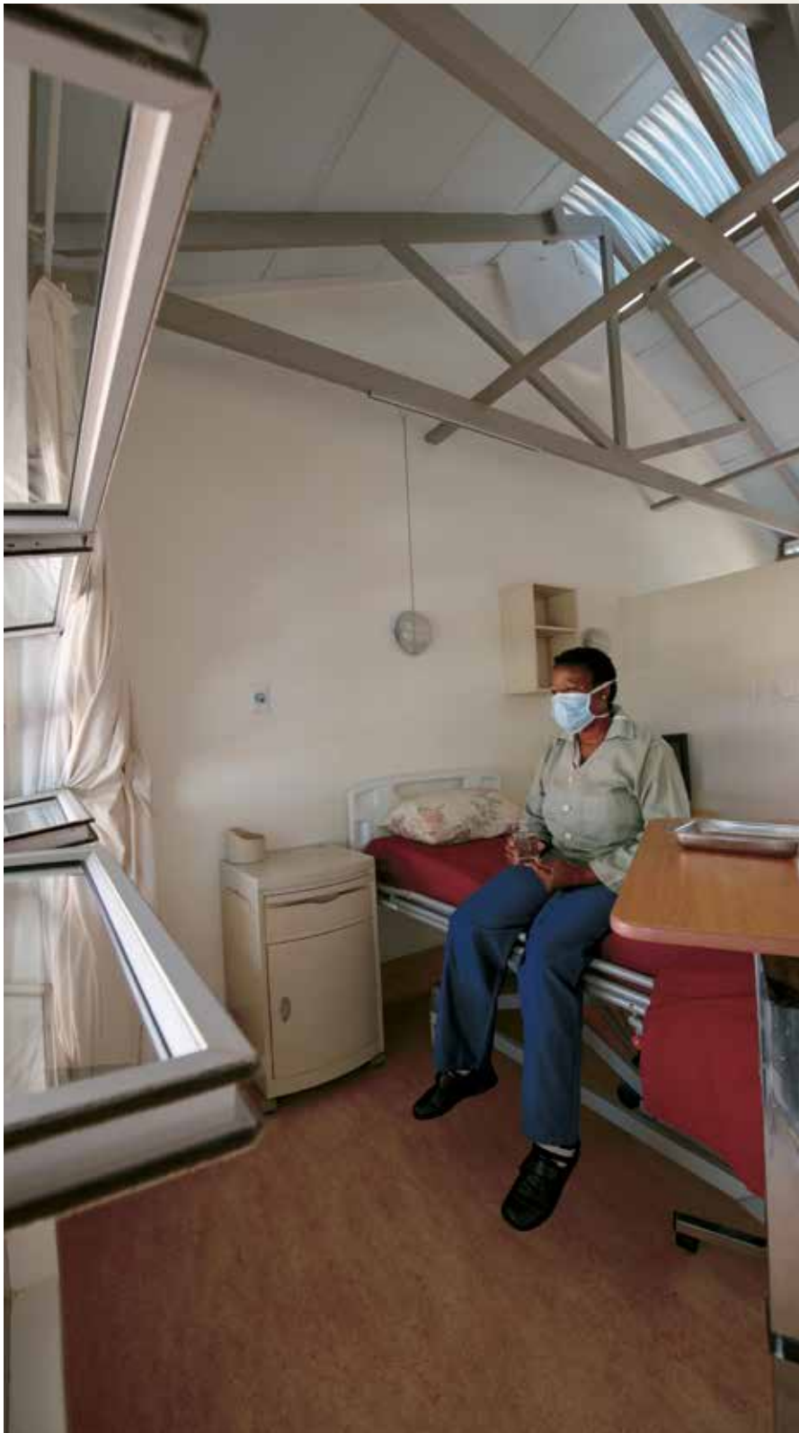
Single rooms for patients with infectious diseases such as tuberculosis are fitted with multiple windows that can open to maximise the movement of air. Here, the warm air will rise to transport potentially infectious organisms through openings in the roof.
