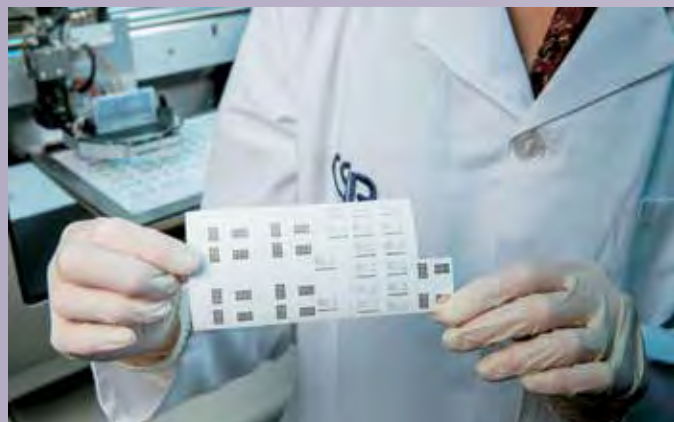
Examples of silver inkjet-printed paper-based sensing electrodes.
