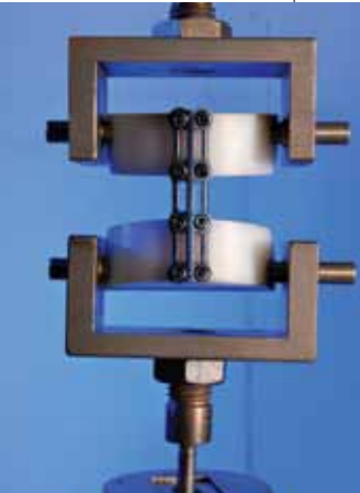
Fatigue testing of a titanium vertebrae plate used for biomedical implants
