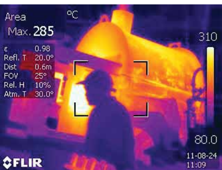
Thermal image, taken at one of the participating foundries, shows areas of heat loss on an aluminium casting furnace.
