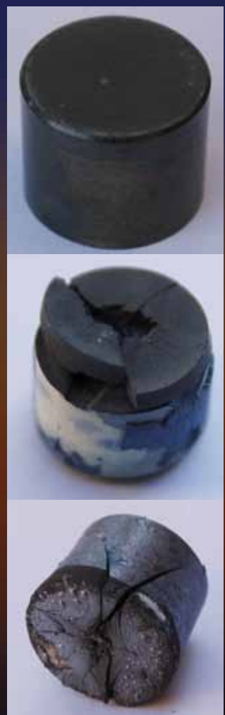
Pictured top is an industrial diamond in good condition, while the two images below show extreme forms of deterioration after laser heating.
