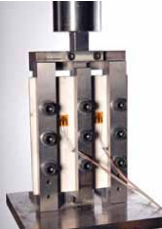
Shear testing of material for South Africa's SKA project (material qualification tests)
