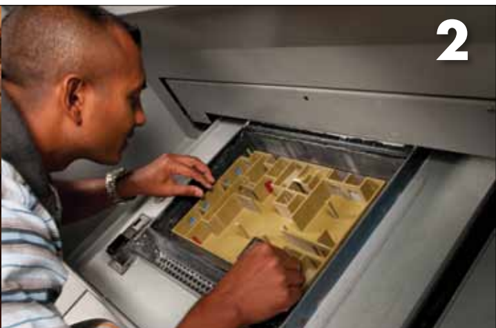
A model is built from a high-performance composite powder, after which post-processing commences.
