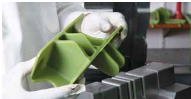
A wax mould of an aircraft part. A face coat as well as a refractory stucco, followed by layers of back-up refractory coats, will cover the final wax assembly. It will be dried completely before the wax can be removed from the formed shell, into which titanium will be cast.
