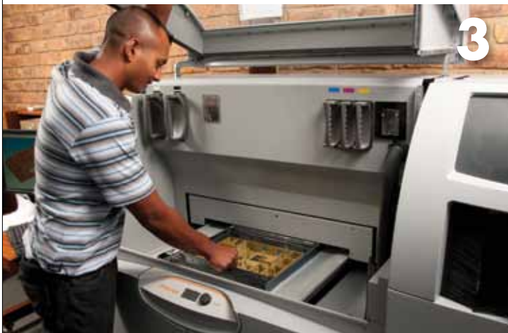
Removal of powder allows for final preparation of the model.
