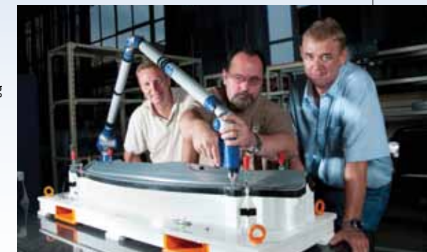
Hansie Pretorius, manager, CSIR laser-enabled manufacturing, right, with Morné Kleinhans, left, and Pieter Bonthuis of MA Automotive Tool and Die, positioning a robotic arm that is used as a tool to align measurements for cutting.
