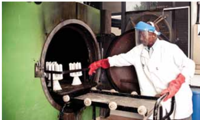
CSIR technical assistant Sam Papo removing casting moulds from the wax melting oven.
