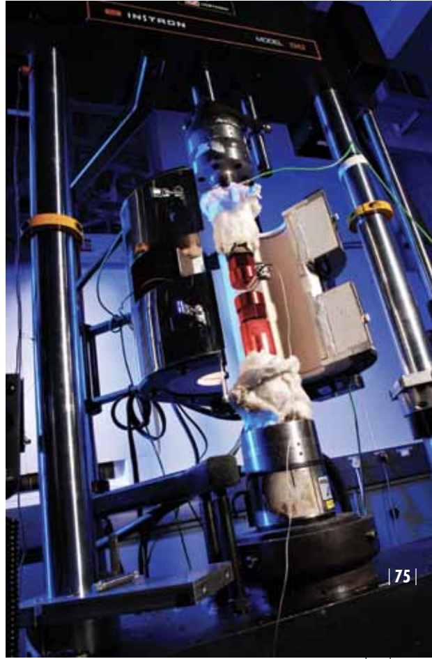
High-temperature tensile testing of turbine-blade material
