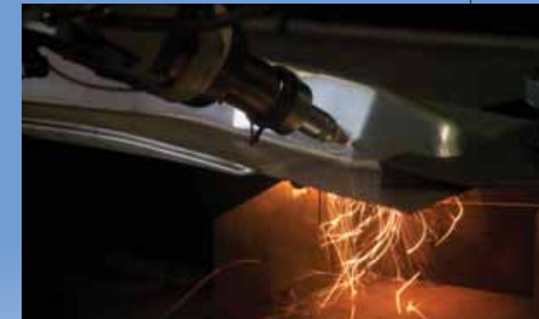
The three-dimensional laser cuts a Maserati part for MA Automotive Tool and Die, a client in the automotive sector.
