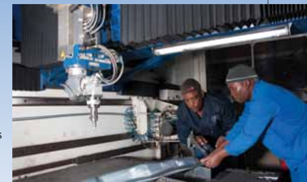
CSIR operators Jacob Mojela, right, and colleague Andrew Madi are seen here laying out the component for laser 3D cutting.
