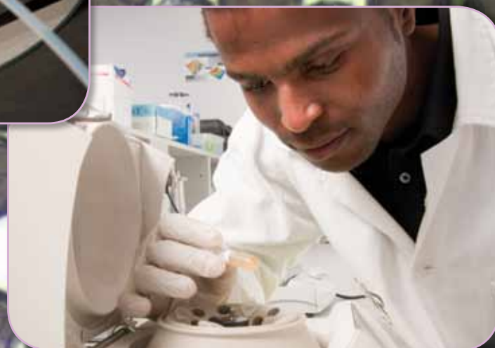
Microfluidics researcher Mesuli Mbanjwa separates manufactured microparticles from oil using a centrifuge.
