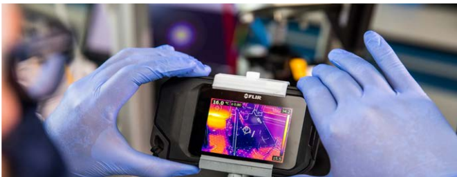
Above: Thermal imaging systems assist engineers to verify opto-mechanical designs and fibre splices for high power laser applications.
