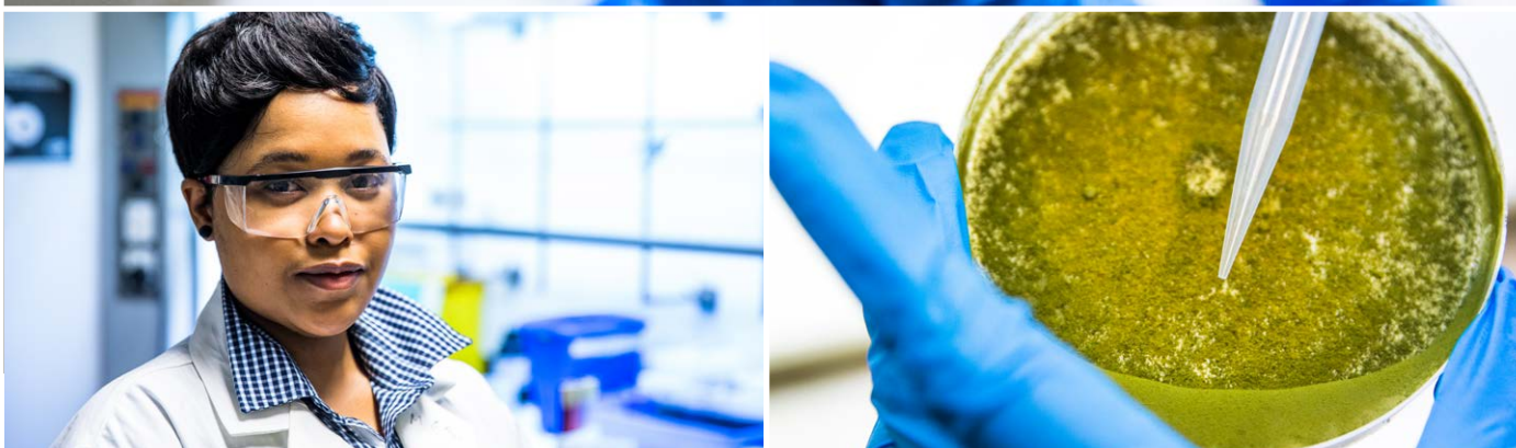
Above: CSIR project leader and chemical engineer Thulisile Nkomzwayo using colorimetric analysis to determine the concentration of kojic acid in a prepared sample. Below (right): An agar plate with the fungal strain used to synthesise kojic acid.
