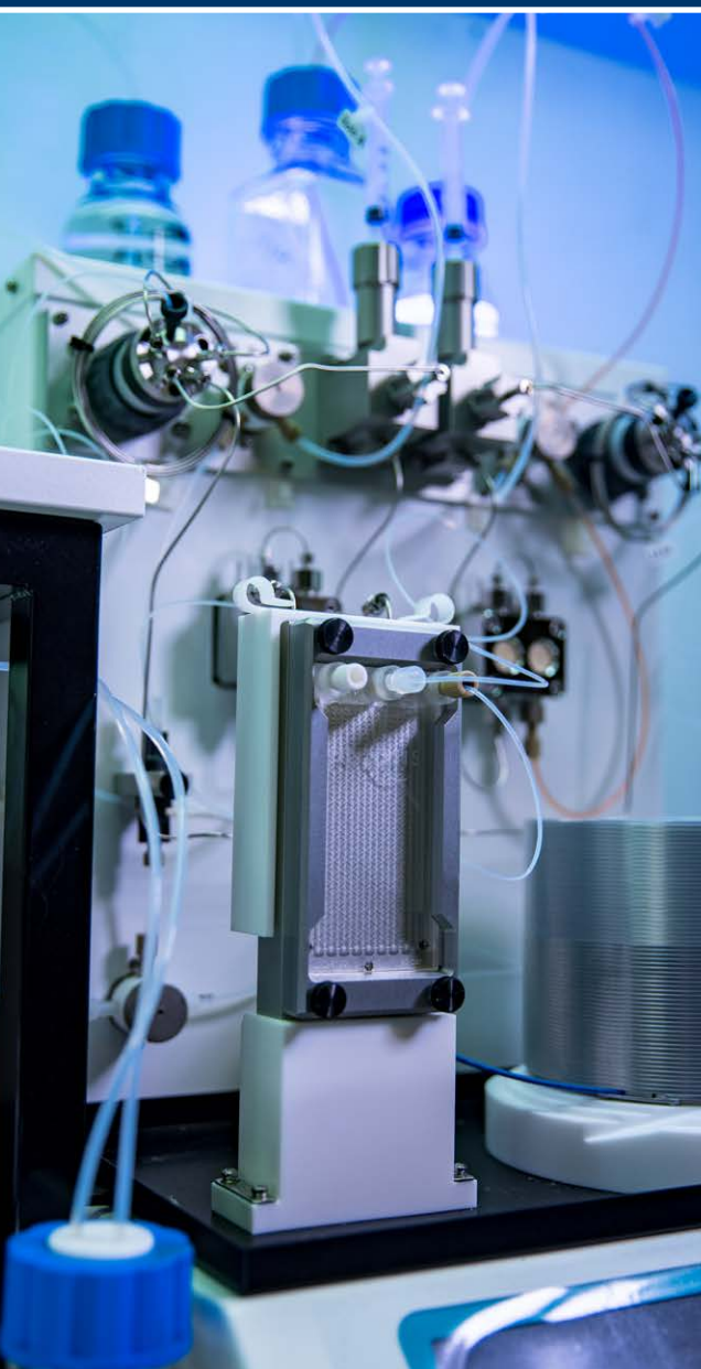
A UniQis FlowSyn Maxi reactor, highlighting the microfluidic mixing chip.
