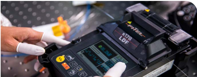
Above and below: The Photonics Prototyping Facility has access to a range of equipment to support the splicing of standard to large diameter optical fibres for laser transmission and high power fibre laser fabrication.
