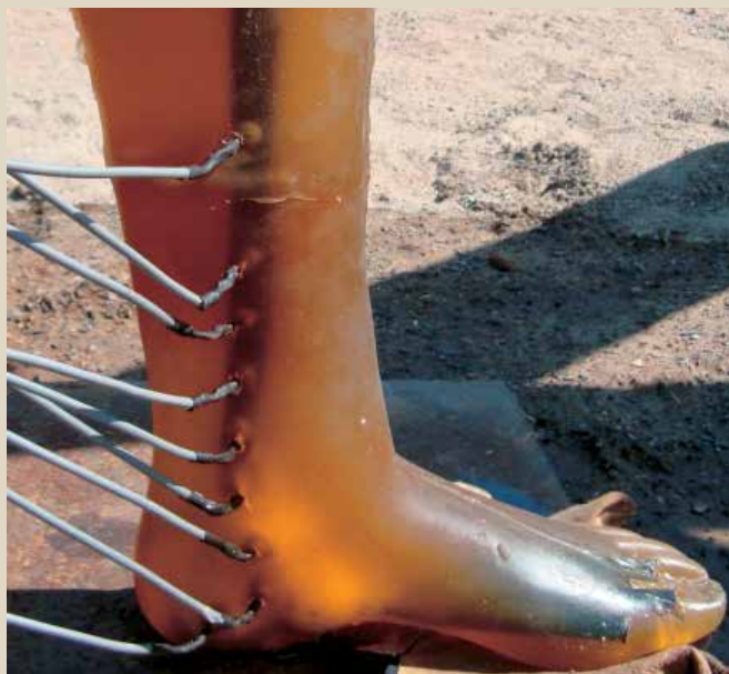
The Frangible Surrogate Lower Limb is a research tool developed by the CSIR to research the impact of antipersonnel mines on lower limbs. Many similar devices exist but the CSIR lower limb is unique in that shock wave velocities and their attenuation through the lower limb can be estimated.
