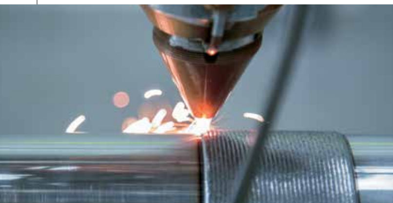
CSIR metallurgist Corney van Rooyen monitors the concast roll cladding process (left). The service life of foot rolls such as those shown above can be increased by up to 300 percent with the use of laser technology.
