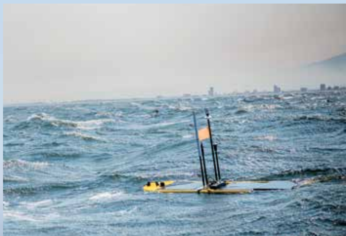
Unmanned marine vehicle fitted with an active sonar system on deployment between Dassen and Robben Islands.
