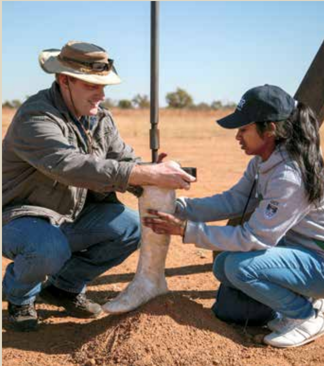
The surrogate lower leg device is used to characterise the effectiveness of mine-resistant boots used in humanitarian de-mining operations. Antipersonnel mines remain a significant scourge in countries with a history of conflict causing much trauma to citizens of these nations.
