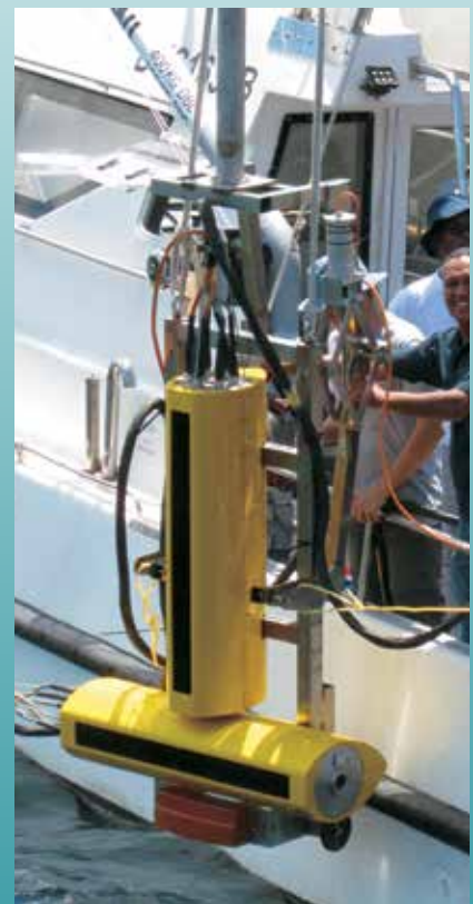
Researchers lowering a sea-going prototype of the CSIR's 3D underwater imaging system during tests.
