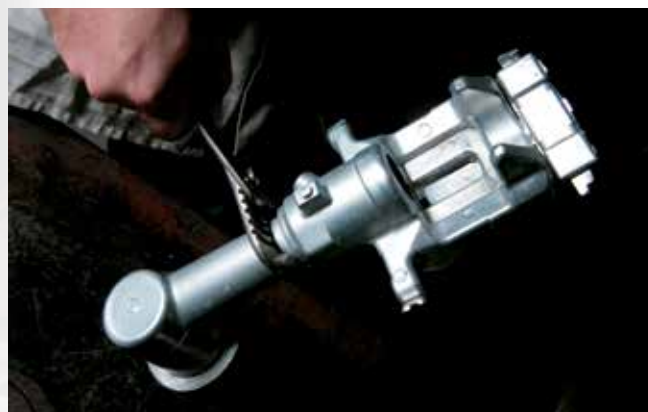
An automotive component (brake calliper) produced in aluminium alloy A356 with the CSIR rheo-high pressure die casting process.
