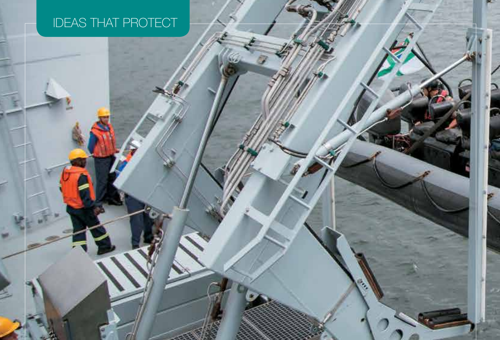
The CSIR-developed wave compensating hydraulic davit system enables deployment of smaller vessels from a moving ship.
