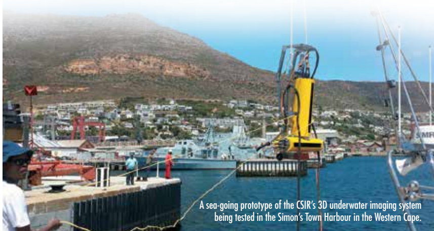
Researchers lowering a sea-going prototype of the CSIR's 3D underwater imaging system during tests.
