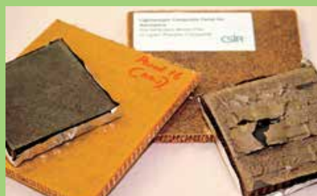
Natural fibre-reinforced sandwich panels for non-load-bearing applications with smaller samples which have undergone fire testing.
