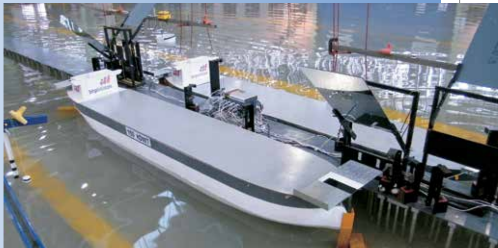
Scaled physical model study of a ship at berth at an iron ore jetty. The ship motions, forces on mooring lines and the force of the ship on the jetty fenders are being determined while the waves impact on the ship.
