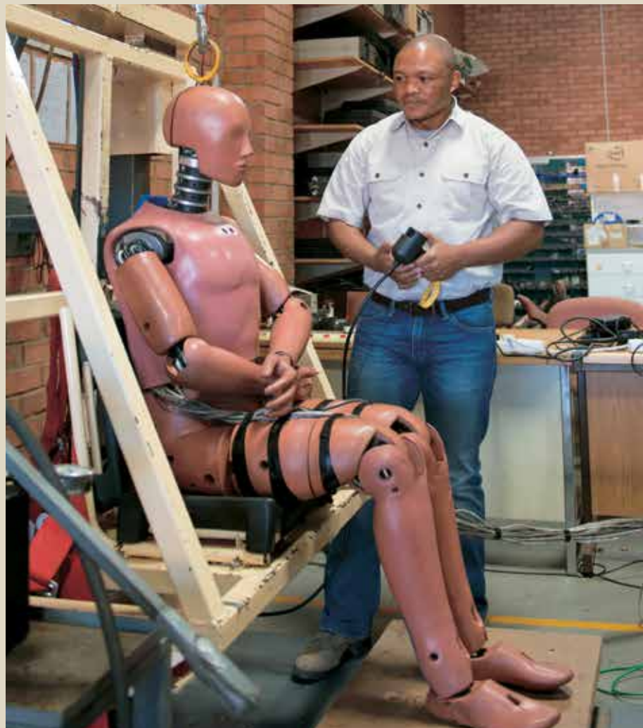
Anthropomorphic test devices – better known as crash test dummies – are installed in a human drop test rig which was designed by the CSIR. Various impact sensors installed in the dummies, as well as high-speed cameras, are used to collect data during tests to evaluate potential injury due to impact caused by an explosive.
