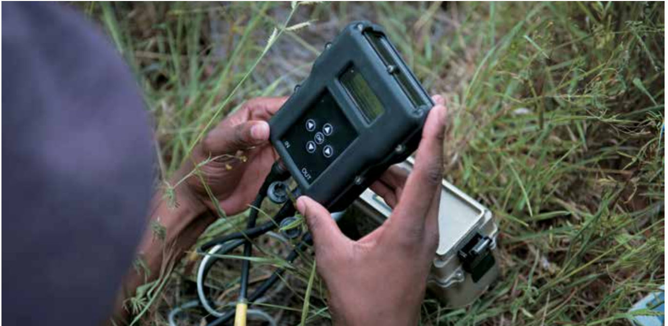
The CSIR-developed power management device weighs less than 500 g and is just bigger than an average male soldier's hand. It has passed the MIL-STD-810F environmental tests, proving its durability for long-term field deployment.
