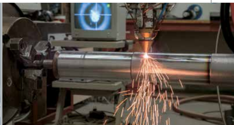
CSIR metallurgist Corney van Rooyen monitors the concast roll cladding process (left). The service life of foot rolls such as those shown above can be increased by up to 300 percent with the use of laser technology.
