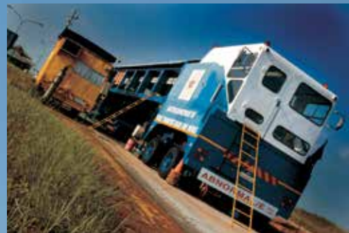
The HVS Mk IV owned by the Gauteng Department of Roads and Transport in operation in the field, testing ultra thin concrete test sections.
