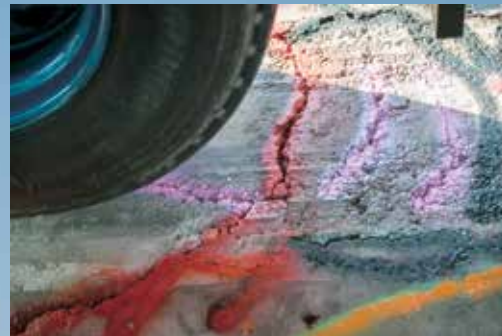
Road cracking failures caused by accelerated testing of the HVS.
