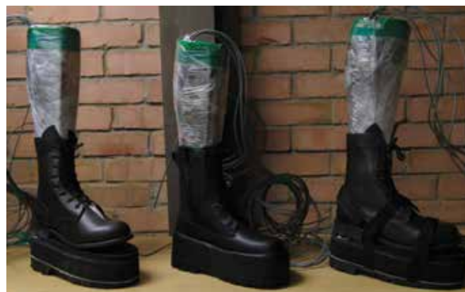
Surrogate lower legs with mine boot concepts fitted – ready for explosive testing.
