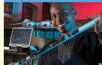
Josias Nonyama, CSIR electronic engineering technologist, holding a receiver printed circuit board housed in a pipe-like probe.
