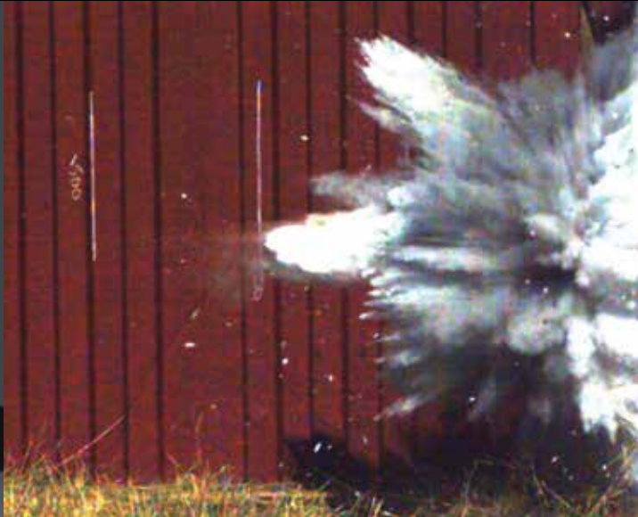
A single frame showing the use of a Quarter cap used in a disruption from 3.1 m
