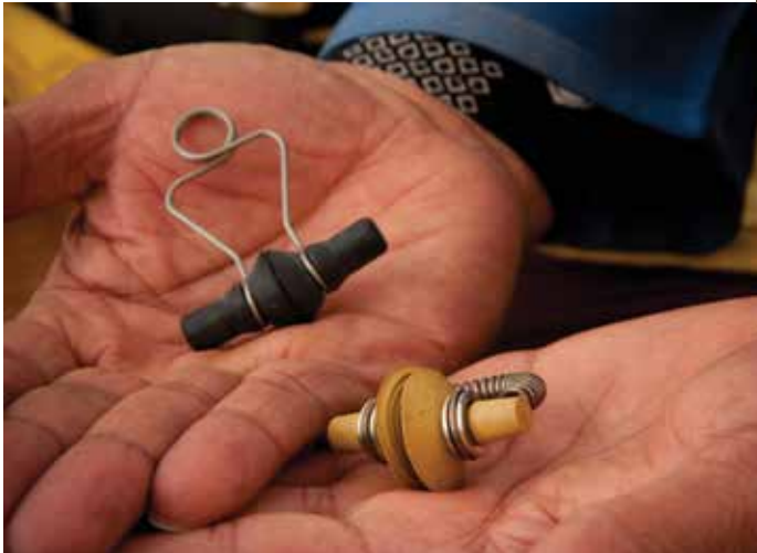
CSIR innovations in mining safety are a nose-clip, used in self-contained, self-rescuers and an electronic sounding device to detect loose overhead rocks after blasting.
