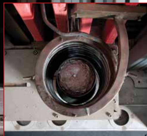
A molten alloy as viewed from above (inserted) during rheocasting at the CSIR's facilities.
