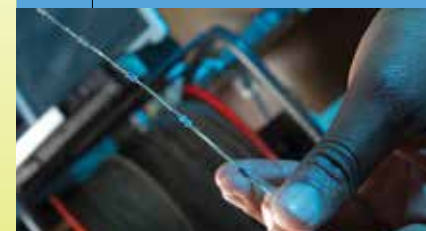
A receiver of the borehole radar system which measures reflections from targets that are illuminated by the transmitter.
