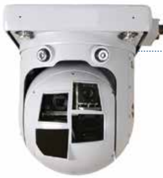
The CoroCAM along with an FLIR product mounted inside a gimbal that is attached to a helicopter. Some power utilities find such a gimbal mounting handy especially when inspecting remote cable lines. This allows them to inspect thousands of km of cable in a much shorter time than would have been possible if done manually.
